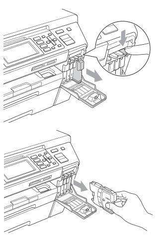
Open the new ink cartridge bag for the color shown on the LCD, and then take out the ink cartridge.
