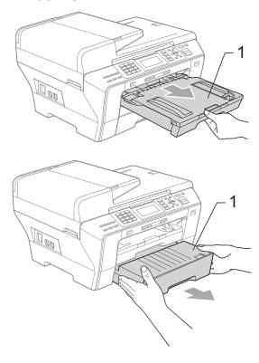
Pull out the jammed paper (1) and press **Stop/Exit**.
