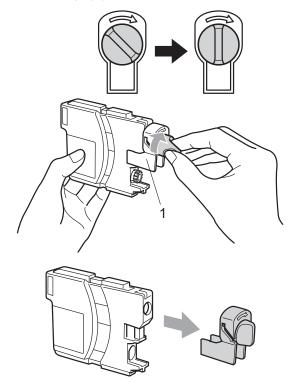
Each color has its own correct position. Insert the ink cartridge in the direction of the arrow on the label.
