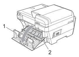
3 Clean the Paper Pick-up Roller (1) with isopropyl alcohol on a cotton swab.
