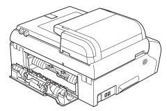
6 Lift the scanner cover (1) from the front side of the machine until it locks securely into the open position. Make sure that there is no jammed paper left inside the machine.
