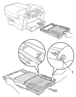
Open the paper tray cover and adjust the paper length guide (1) for the paper.
