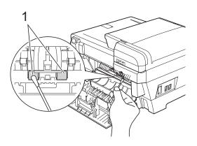
(MFC-5890CN and MFC-5895CW) Close the Jam Clear Cover properly.
