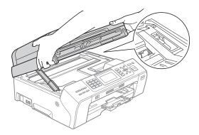
If ink gets on your skin or clothing immediately wash it off with soap or detergent. Lift the scanner cover to release the lock (1). Gently push the scanner cover support down (2) and close the scanner cover (3) using both hands.
