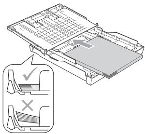
Gently adjust the paper side guides to fit the paper with both hands. Make sure the paper side guides touch the sides of the paper.
