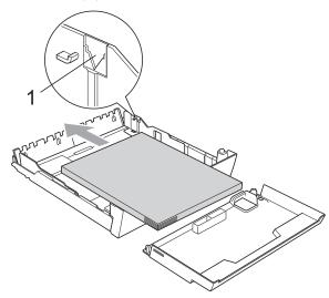
Gently adjust the paper side guides with both hands to fit the paper stack. Make sure the paper side guides touch the sides of the paper.
