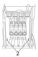
If you are not able to find the green protective part, DO NOT remove the ink cartridges before shipping. It is essential that the machine be shipped with either the green protective part or the ink cartridges in position. Shipping without them will cause damage to your machine and may void your warranty.
