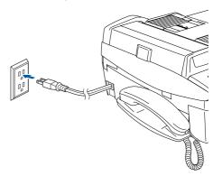
Connect the telephone line cord. Connect one end of the telephone line cord to the jack on the machine marked LINE and the other end to a modular wall jack.
