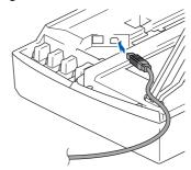
Carefully route the USB cable through the trench and out the back of the machine as shown below.
