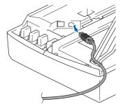
10 Carefully route the USB cable through the trench and out the back of the machine as shown below.
