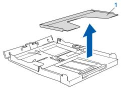
Press and slide the paper guide (1) to fit the paper width.
