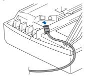
Carefully route the network cable through the trench and out the back of the machine as shown below.
