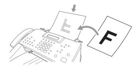
The ADF (automatic document feeder) can hold up to 30 Pages, feeding each one individually through the machine. Use standard (17 lb–24 lb) paper when using the ADF. If you're using heavier paper, feed each sheet individually to prevent paper jams.
