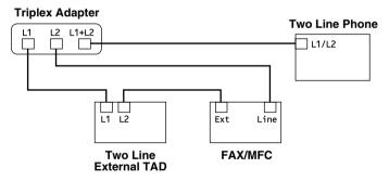
You can keep two-line telephones on other wall outlets as always. There are two ways to add a two-line telephone to the machine's wall outlet. You can plug the telephone line cord from the two-line telephone into the L1+L2 jack of the triplex adapter. Or, you can plug the two-line telephone into the TEL jack of the two-line TAD.
