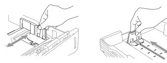
Fan the paper well. Load paper in the paper cassette. Press down on the paper to flatten it in all four corners, keeping the paper level below the guide. The cassette can hold up to 250 sheets of 20 lb (75g/m<sup>2</sup>) paper.
