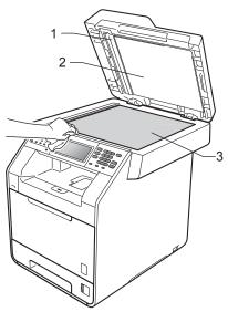
4 In the ADF unit, clean the white bar (1) and the glass strip (2) underneath it with a soft lint-free cloth moistened with water.
