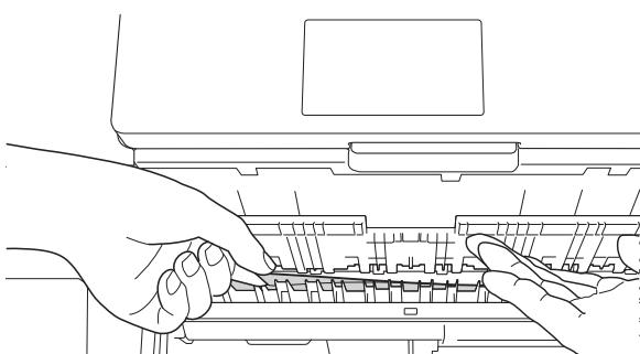
6 Using both hands, use the finger holds on each side of the machine to lift the scanner cover (1) into the open position.
