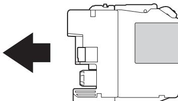
6 Gently push the back of the ink cartridge marked PUSH until it latches, and then close the ink cartridge cover.
