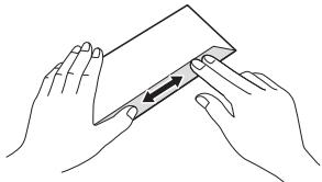
2 Gently press and slide the paper side guides to fit the paper size.
