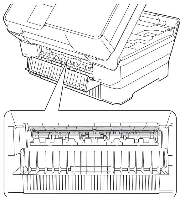
13 Close the inside cover and Jam Clear Cover. Make sure the covers are closed completely.
