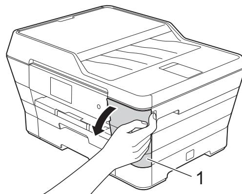
2 Press the lock release lever as shown to release the cartridge color indicated on the Touchscreen. Remove the cartridge from the machine.
