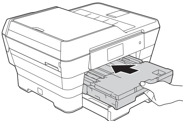
15 Pull out the paper support (1) until it locks into place, and then unfold the paper support flap (2).
