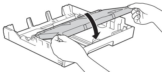
2 Gently put the paper into the paper tray printing surface face down. Check that the paper is flat in the tray.
