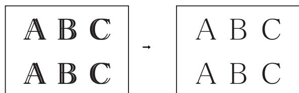
When the print alignment is not adjusted properly, text looks blurry like this.
