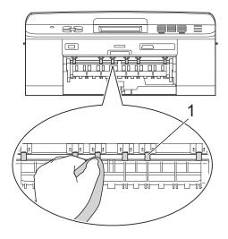
3 Lift the Jam Clear flap (2), and then clean the back side of the Paper Feed Rollers (1) with a soft lint-free cloth moistened with water.
