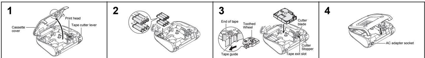
**1** Open the cassette cover by pressing the indicated area at the back of the machine. If a tape cassette is already installed, remove it by pulling it straight up. Also, if batteries are already installed, remove them.
