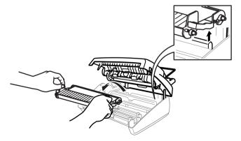
**4** To clean your machine's print head, wipe the print head with a lint-free cloth that is dry or lightly moistened with isopropyl alcohol.
