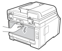
2 <For printing envelopes only> Pull down the two grey levers, one on the left-hand side and one on the right-hand side, toward you as shown in the illustration below.
