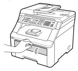
Using both hands, slide the manual feed slot paper guides to the width of the paper that you are going to use.
