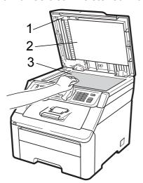
3 In the ADF unit, clean the white bar (1) and the scanner glass strip (2) underneath it with a soft lint-free cloth moistened with water.
