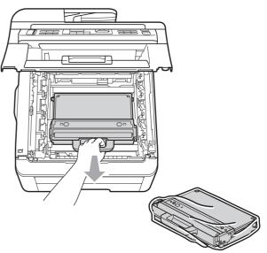
9 Reinstall the belt unit back in the machine.
