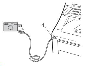
Turn on the camera. Make sure your camera is in PictBridge mode. When the machine has recognized the camera, the LCD shows the following message.
