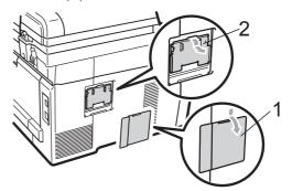
Unpack the SO-DIMM and hold it by its edges.
