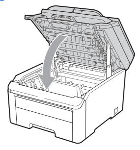
12 Put the waste toner box and one drum unit and toner cartridges assembly in the Styrofoam piece.
