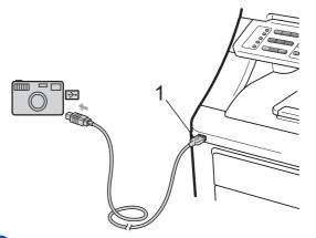
Turn on the camera. Make sure your camera is in PictBridge mode. When the machine has recognized the camera, the LCD shows the following message depending on which mode the machine is in:
