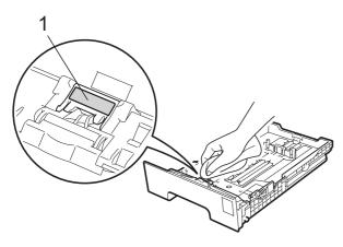
4 Wipe the two pick-up rollers (1) inside of the machine to remove dust.
