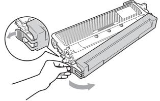
8 Put the new toner cartridge firmly into the drum unit until you hear it lock into place.
