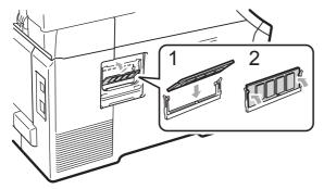
6 Put the metal (2) and then the plastic (1) SO-DIMM covers back on.
