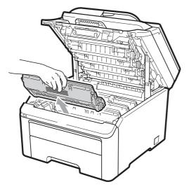
Push down the green-labelled lock lever (1) and take the toner cartridge out of the drum unit.
