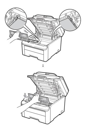
10 Reinstall the original packing material into the machine.
