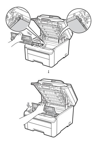
9 Slide each drum unit and toner cartridge assembly into the machine. Make sure that you match the toner cartridge colour to the same colour label on the machine. Repeat this for all the drum unit and toner cartridge assemblies.
