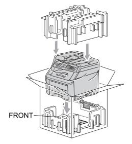
15 Put the power cord, and the three remaining drum unit and toner cartridge assemblies into the Styrofoam pieces as shown in the illustration.
