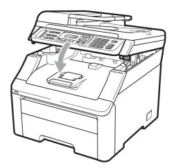
• When the top cover is open, you cannot open the scanner.
