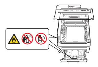
DO NOT use a vacuum cleaner to clean up scattered toner. Doing this might cause the toner dust to ignite inside the vacuum cleaner, potentially starting a fire. Please carefully clean the toner dust with a dry, lint-free soft cloth and dispose of it according to local regulations.
