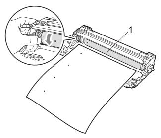
7 When you have found the mark on the drum that matches the print sample, wipe the surface of the OPC drum with a dry cotton swab until the dust or glue on the surface comes off.
