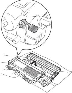
9 Put the drum unit and toner cartridge assembly back in the machine.
