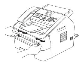
7 Using both hands, put one piece of A4 or Letter size paper in the manual feed slot until the top edge of the paper touches the paper feed roller. When you feel the machine pull in the paper, let go. The machine will start the Drum Cleaning process.
