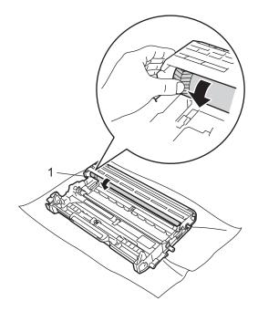
7 When you have found the mark on the drum that matches the print sample, wipe the surface of the OPC drum with a dry cotton swab until the dust or glue on the surface comes off.
