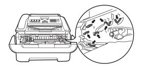
3 Clean the corona wire inside the drum unit by gently sliding the green tab from left to right and right to left several times.
