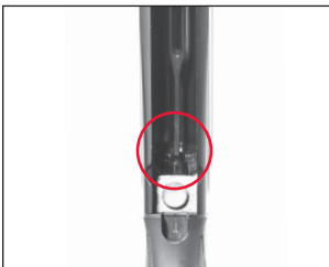
Guide the bolt slide link into its socket in the recoil spring follower.
