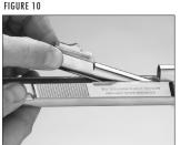
Lift out the barrel.
