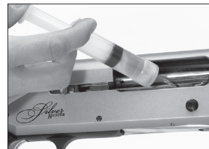
Occasionally place a drop of light gun oil on the rails inside the receiver.
