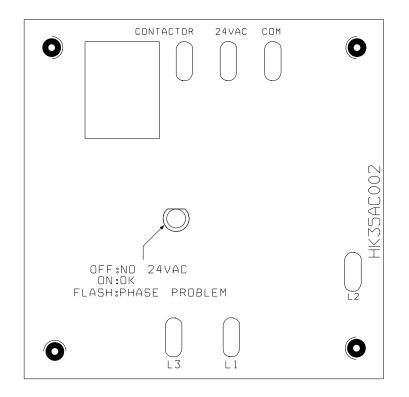
Fig. 31—CES0130075 3–Phase Monitor Board
