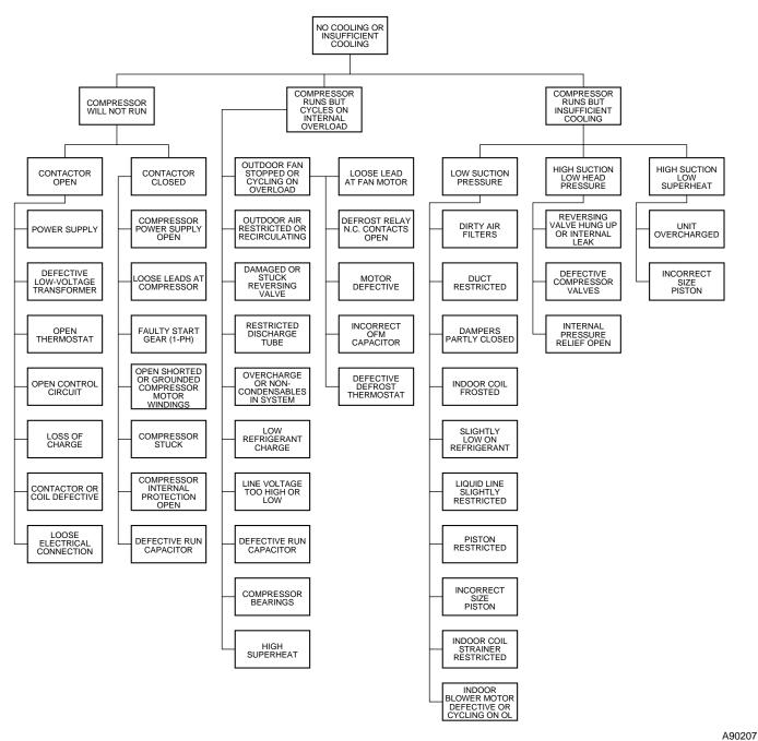
Fig. 53—Heat-Pump Troubleshooting Chart — Cooling Cycle
