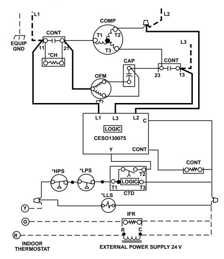
Fig. 32—CESO130075 3–Phase Monitor Wiring Diagram
