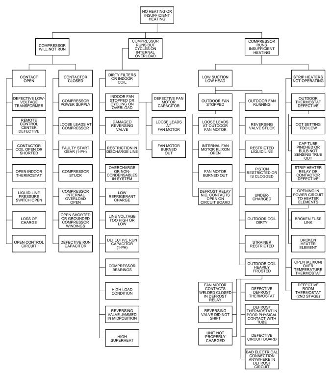
Fig. 54—Heat-Pump Troubleshooting Chart — Heating Cycle
