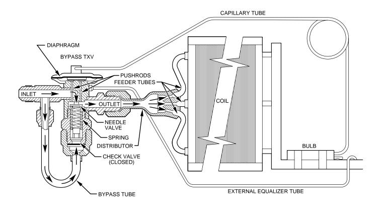
Fig. 49—TXV in Cooling Mode
