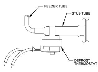
Fig. 23—Defrost Thermostat Location
