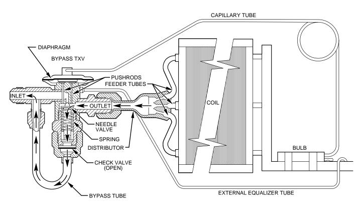
Fig. 50—TXV in Heating Mode
