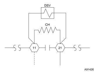
Fig. 18—Wiring for Single-Pole Contactor
