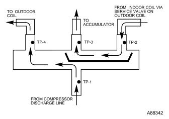
Fig. 47—Reversing Valve (Cooling Mode or Defrost Mode, Solenoid Energized)
