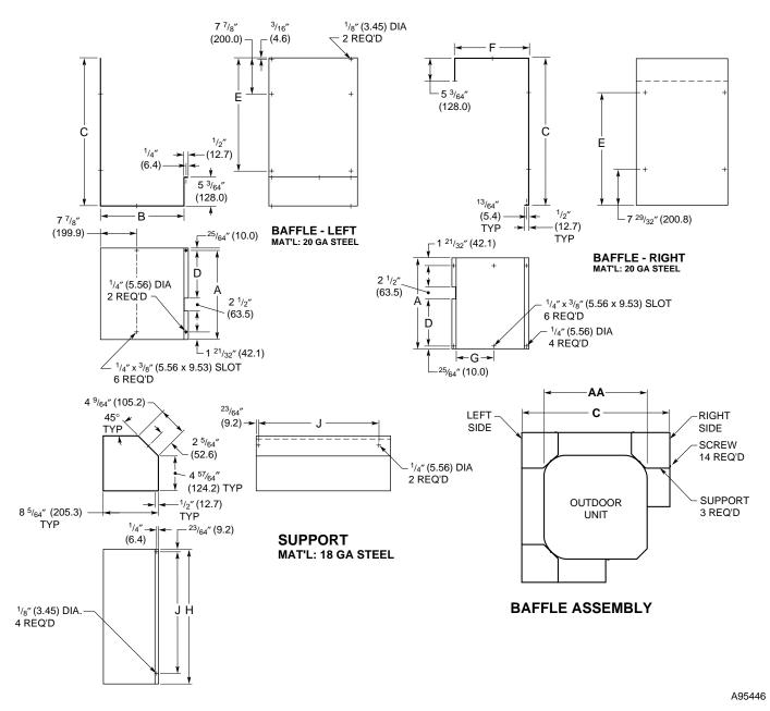
Fig. 2—Wind Baffle Construction for Cube Units
