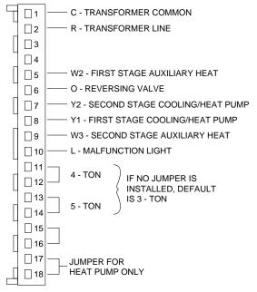
Fig. 37—Header-Pin Housing
