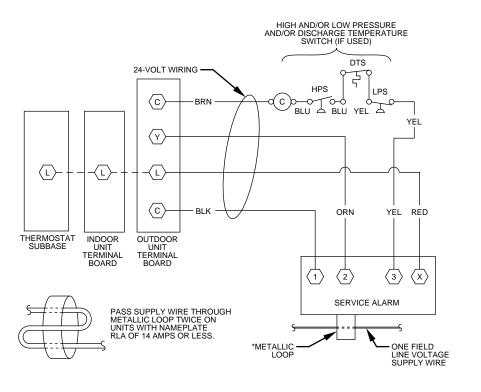
Fig. 25—Service Alarm Wiring Connections
