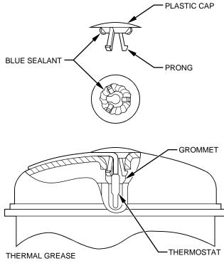
Fig. 30—Location of Discharge Thermostat
