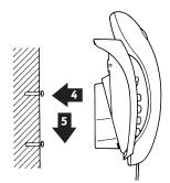
Handset hook Keeps the handset in place when the Decor 310 is wall mounted.
