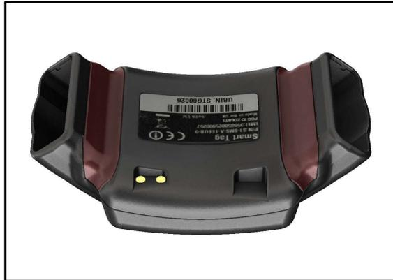
The Locking Plates will be secured in position when the Strap is inserted into the Smart Tag 5 XB, they protect the strap from being released without physical damage being created for evidence gathering purposes.
