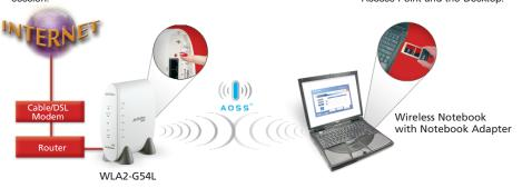
The Wireless Distribution System (WDS) or Bridge/Repeater Mode allows the AirStation to wirelessly communicate with other Buffalo AirStation Access Points (Base Stations) that support WDS. The AirStation 54 Mbps\* Standard Bridge Base Station supports communication with up to six other Buffalo Bridge APs for point-to-point or point-to-multi-point communication and to cover dead zones in WLANs
