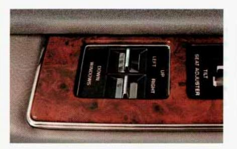
To lower the window, pull back on the switch. The window will lower as long as the switch is held. To raise the window, push the switch forward.
