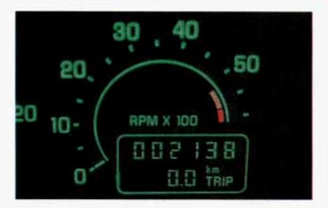
The tachometer tells you how fast the engine is going. It displays engine speed in revolutions per minute (RPM). As engine speed increases, the bars light up on the tachometer display. Each bar represents 100 RPM. Do not operate your car's engine in the red line range. If you do, you can cause severe engine damage.
