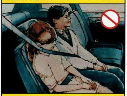
Here two children are wearing the same belt. The belt can't properly spread the impact forces. In a crash, the two children can be crushed together and seriously injured. A belt must be used by only one person at a time.
