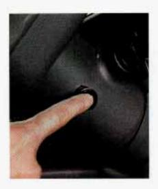
Press the button in to make your front and rear turn signal lights flash on and off.
