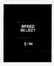
By pushing the E/M (English/Metric) button, the digital display can be changed to read English (miles) or metric (kilometers).
