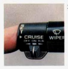
Push in set the button at the end of the lever and release it. (The "CRUISE" light on the instrument panel will come on.)
