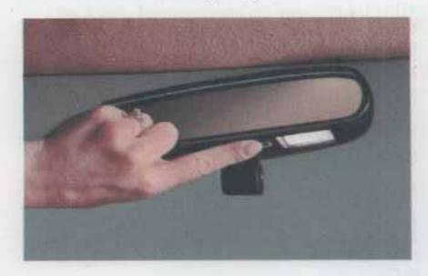
Turn on the front seat reading lights by pressing the switch located on the inside rearview mirror.
