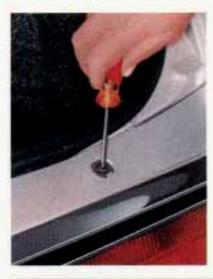
Using a Phillips® screwdriver remove the long screws.
