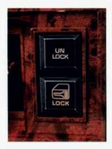
Push the power door lock switch to lock or unlock both doors at once.
