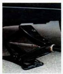
Position the jack under the vehicle. There is a notch in the frame near each of the wheels. Fit the lift head of the jack into the notch nearest the wheel with the flat tire.
