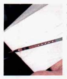
To Check Engine Oil: Pull out the dipstick and clean it with a paper towel or cloth, then push it back in all the way. Remove it again, keeping the tip lower.
