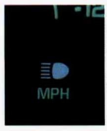
To change the headlights from low beam to high or high to low, pull the turn signal lever all the way toward you. Then release it. When the high beams are on, a blue light on the instrument panel also will be on.
