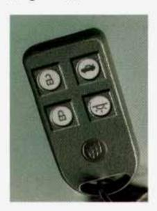
If your Buick has this option, you can lock and unlock your doors or unlock your trunk from up to 15 feet (5 m) away using the key chain transmitter supplied with your vehicle
