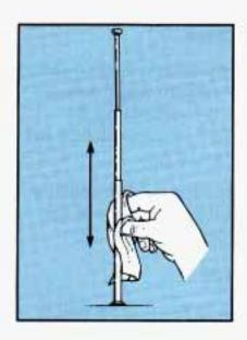
Wipe cloth over the mast sections, removing any dirt.
