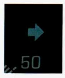
A green arrow on the instrument panel will flash in the direction of the turn or lane change.
