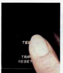
Press and hold the Test button with your car in Park or Neutral. This test makes sure all your bulbs and bar graph segments are working. If any are not working, have the bulbs replaced.
