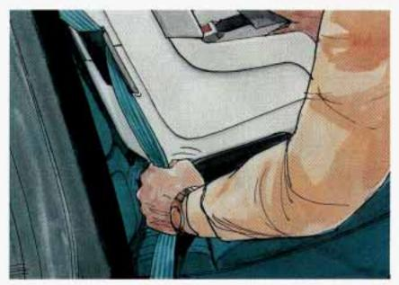
To tighten the belt, feed the lap belt back into the retractor while you push down on the child restraint.
