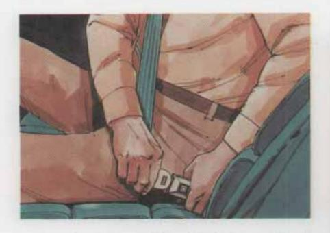
Pick up the latch plate and pull the belt across you. Don't let it get twisted. 2. Push the latch plate into the buckle until it clicks.
