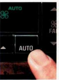
When the system is set for automatic, air will come from the floor outlets, the instrument panel outlets or both. Fan speed will vary (unless a blower LO or HI button has been pushed) as the system gets to and maintains the temperature setting you have selected.
