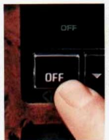
When the system is off, the ventilation system will allow air to flow through your Buick when the vehicle is moving. The system will try to keep the air at the chosen temperature, unless it is very hot or very cold outside.
