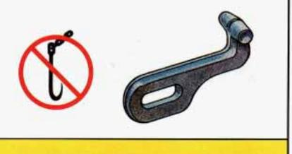
When your vehicle is being towed, have the ignition key off. The steering wheel should be clamped in a straight-ahead position, with a clamping device designed for towing service. Do not use the vehicle's steering column lock for this. The transaxle should be in Neutral and the parking brake released.
