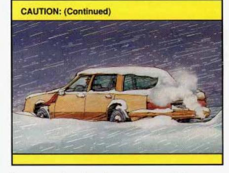
Run your engine only as long as you must. This saves fuel. When you run the engine, make it go a little faster than just idle. That is, push the accelerator slightly. This uses less fuel for the heat that you get and it keeps the battery charged. You will need a well-charged battery to restart the vehicle, and possibly for signaling later on with your headlights. Let the heater run for awhile.
