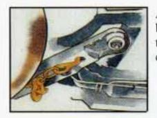
Attach "T" hook chains behind the front wheels into the bottom of slots of the cradle rails on both sides.
