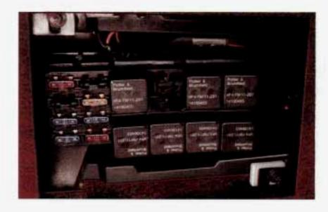
There is also a fuse block that is located on the right side of the console under a carpeted panel cover. Remove the cover to access these fuses.
