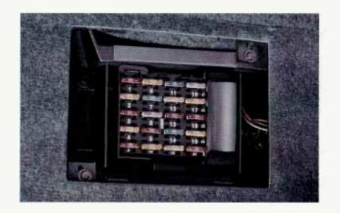
There are two fuse block areas inside your vehicle. One is located on the left side of the console under a carpeted panel cover. Remove the cover to access the fuses.
