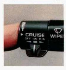
Push the button at the end of the lever, then release the button and the accelerator pedal. You'll now cruise at the higher speed. Here's the second way to go to a higher speed:
