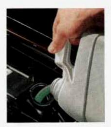
Fill the radiator with the proper mix, up to the base of the filler neck.
