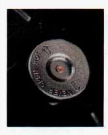
Then replace the pressure cap. Be sure the arrows on the pressure cap line up like this.
