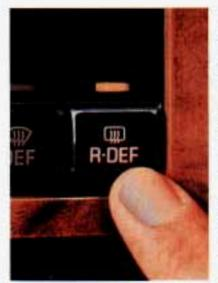
The lines you see on the rear window will warm the glass. Press the button to start warming your window. After 10 minutes, it will go off by itself, or by pressing the button again will shut it off. If you need additional warming time, push the button again.
