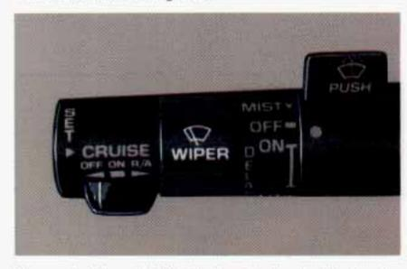
You control the windshield wipers by turning the band marked "WIPER."
