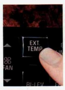
Press this button to display outdoor temperature. Press it again to return to the regular display. The outside temperature will display if the system is "OFF".
