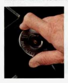
1. You can remove the radiator pressure cap when the cooling system, including the radiator pressure cap and upper radiator hose, is no longer hot.
