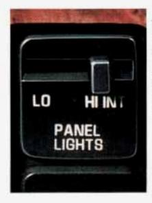
The instrument panel light brightness can be adjusted when the parking or headlights are on. Slide the lever toward HI to make them brighter; toward LO to dim them. Push the lever to INT to turn on the interior lights.
