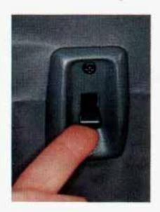
To fold a seatback forward, push the seatback toward the rear as you lift this latch. Then the seatback will fold forward. The latch must be down for the seat to work properly.
