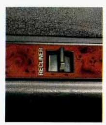
If you have the power option, it works with the switch located on the side of the seat.
