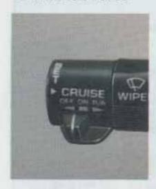
With Cruise Control, you can maintain a speed of about 25 mph (40 km/h) or more without keeping your foot on the accelerator. This can really help on long trips. Cruise Control does not work at speeds below about 25 mph (40 km/h).
