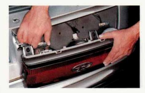
Remove the bulb socket by squeezing the plastic lock and turning it counterclockwise.
