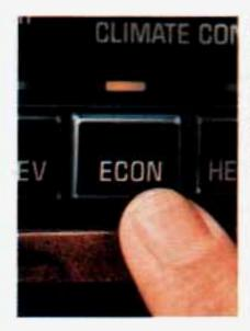
You can use this when you don't need to cool the outside air. The system will work as in the AUTO mode without cooling. The air will come from the instrument panel outlets.
