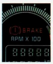
Your Buick's hydraulic brake system is divided into two parts. If one part isn't working, the other part can still work and stop you. For good braking, though, you need both parts working well.
