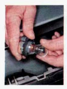
Remove the bulb from the bulb socket by turning it counterclockwise.
