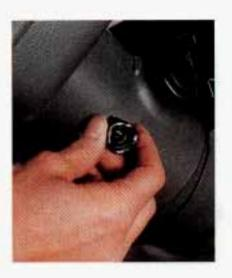
To turn off the flashers, pull out on the collar. When the hazard warning flashers are on, your turn signals won't work.
