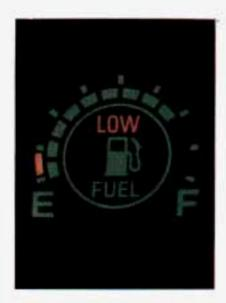
Your fuel gage is a bar graph. When you fill the tank, the bar segments will light up. The fuel gage shows about how much fuel is in your tank. It works only when the ignition is on. When the fuel gage shows only two bar segments the "LOW" light will come on. If the fuel supply is in the one bar segment, the yellow warning bar will flash to remind you to get more fuel soon.
