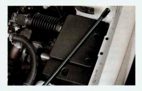
As you face the front of the vehicle, the air cleaner is in the front right section of the engine compartment. There is a filter inside the air cleaner.
