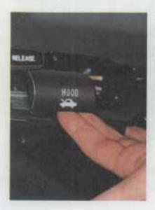
To open the hood, first pull the handle inside the vehicle. It is located on the lower left side of the instrument panel, next to the parking brake release.
