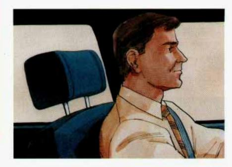
Slide the head restraint up or down so that the top of the restraint is closest to the top of your ears.
