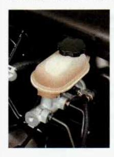
Your brake master cylinder is here. It is filled with DOT-3 brake fluid.
