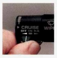
Move the Cruise switch to "OFF." (The "CRUISE" light will go out.)
