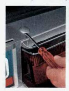
Open the trunk and locate the plastic plugs above each taillamp. Insert a small screwdriver blade into the notch of each of the two plugs and carefully twist the screwdriver to remove.
