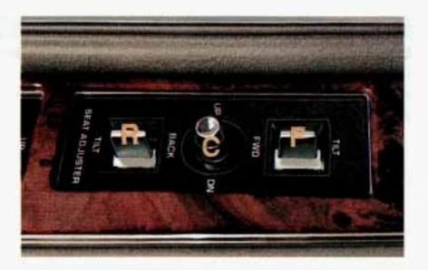
Front Control (F): Raise or lower the front of the seat by holding the switch to the right or left.
