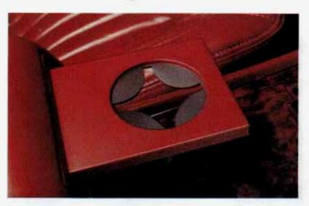
The center console has space for cassette storage, a coinholder and a cupholder. The cupholder is on the front of the storage console. Press on the exposed edge of the cupholder, and it will slide out for use. Press the front edge again, to slide it back to it's storage position.
