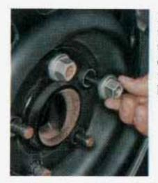
Replace the wheel nuts with the rounded end of the nuts toward the wheel. Tighten each nut by hand until the wheel is held against the hub.
