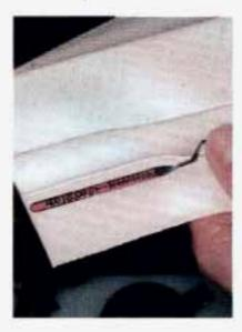
Check both sides of the dipstick, and read the lower level. The fluid level must be in the cross-hatched area.
