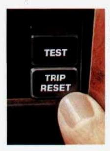
A trip odometer can tell you how many miles you have driven since you last set it back to zero. To reset, push the button.
