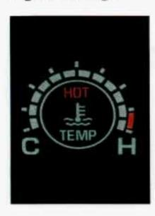
The "HOT" light tells you that your engine coolant has overheated or your radiator cooling fan is not working. The gage also shows the engine coolant temperature. If the gage reading moves into the red area, your engine has overheated. If you have been operating vour vehicle under normal driving conditions, you should pull off the road, stop your vehicle and turn the engine off as soon as possible.
