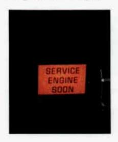
A computer monitors operation of your fuel, ignition and emission control systems. This light should come on when the ignition is on, but the engine is not running, as a check to show you it is working. If it does not come on at all, have it fixed right away. If it stays on, or it comes on while you are driving, the computer is indicating that you have a problem. You should take your vehicle in for service soon.
