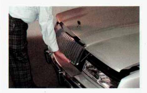
Then go to the front of the vehicle and locate the secondary hood release. It is located under the front edge of the grill. Push up on the secondary hood release lever, then lift up the hood.
