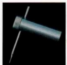
To remove the wire wheel cover, remove the center of the wheel cover by using the wire wheel key wrench.
