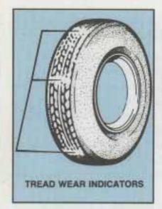
One way to tell when it's time for new tires is to check the treadwear indicators, which will appear when your tires have only 2/32 inch (1.6 mm) or less of tread remaining.
