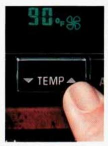
To choose the temperature you want maintained inside the vehicle, press the TEMP ▲ or ▼ for warmer or cooler.
