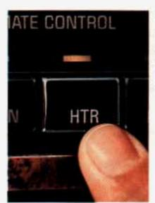
To warm the air, press HTR and adjust the temperature and fan speeds for your comfort. Most of the air will come from the floor outlets.
