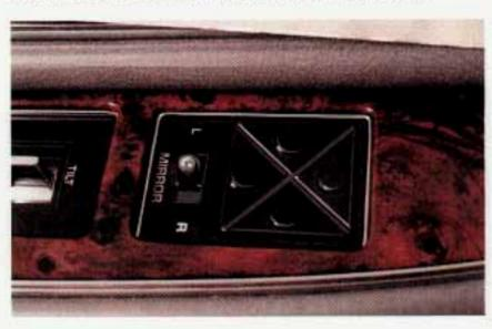
Move the switch to the right (R) or left (L) to choose a mirror. Press any of the four buttons to move the mirror in the direction desired.
