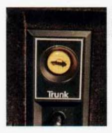
Push the TRUNK button found in the glove box to unlock the trunk.
