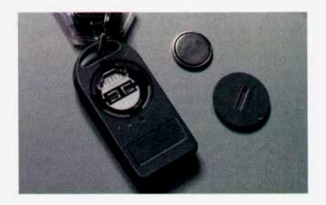
To replace the battery, insert the round end of the door lock key into the slot of the access door on the back of the transmitter. Turn the door one-sixteenth of a turn to the left, and lift it out of the transmitter. Remove the battery and replace it with a Sanyo CR2025 or equivalent. It is important to use the correct size battery. Using the wrong battery may damage the transmitter.
