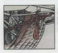
Attach "T" hook chains to the slots in the bottom of the floor pan just ahead of the rear wheels on both sides.
