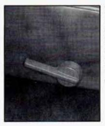
To adjust the seatback, lift the lever on the outer side of the seat and move the seatback to where you want it. Release the lever to lock the seatback. Pull up on the lever and the seat will go to an upright position.
