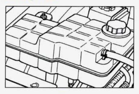
The surge tank is in the engine compartment, directly behind the battery.
