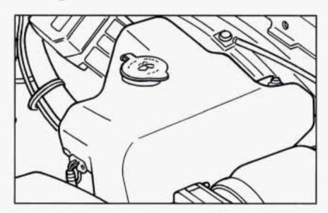
The windshield washer reservoir is located on the driver's side of the engine compartment.
