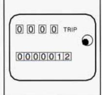
A trip odometer can tell you how may miles you have driven since you last set it to zero. To reset it, press the button.
