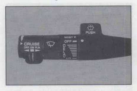
You control the windshield wipers by turning the band with the wiper symbol on it. For a single wiping cycle, turn the band to MIST. Hold it there until the wipers start, then let go. The wipers will stop after one cycle. If you want more cycles, hold the band on MIST longer.
