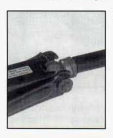
2. Attach the wheel wrench to the bolt at the end of the iack. Rotate the wheel wrench clockwise to slightly raise the lift head.
