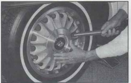
Remove this wheel cover by carefully prying off the center of the cover with the flat end of the wheel wrench.
