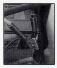
Now connect the black negative (-) cable to the good battery's negative (-) terminal.
