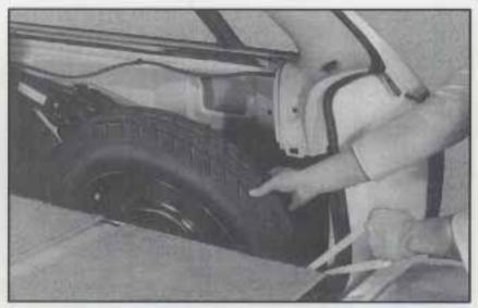
Using the tire lift strap, pull the tire out of the storage well.
