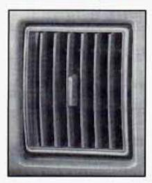
Adjust the direction of airflow by moving the louvered vents.
