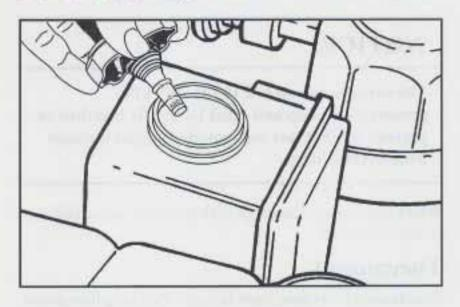
The power steering cap is to the left of the engine fan when you are facing the engine.
