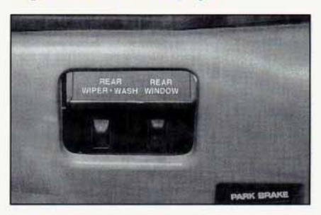
Press the top of the REAR WIPER-WASH switch to turn on the rear wiper. Press the bottom of the switch to turn it off.
