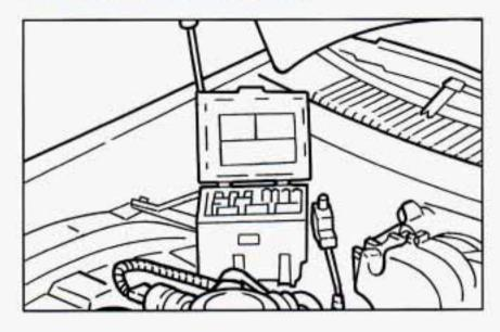
Lift the hood and open the cover to gain access to this fuse block.
