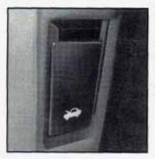
To open the hood, first pull the handle inside the vehicle. It is located on the lower left side of the instrument panel, next to the parking brake.
