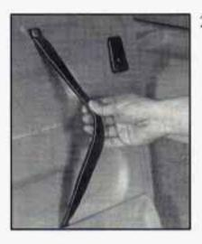
Pull the seatback down using the assist strap, then push down on it to lock it into place.
