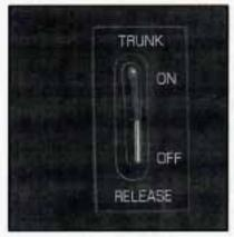
The security switch in the glove box must be ON for the TRUNK button to work.
