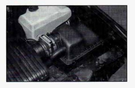
The air cleaner is located on the driver's side of the engine compartment.
