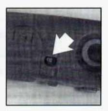
Use a cotton swab and glass cleaner to clean the front and rear photocells that make the electrochromic mirror work.
