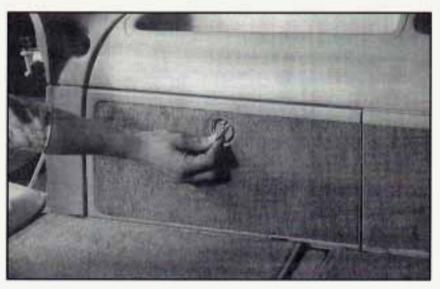
Turn the key to the right to unlock. The key cannot be removed in this position.
