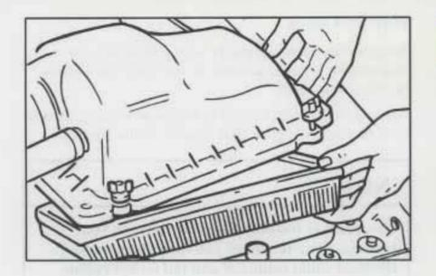
Remove the air filter. Be sure to inspect both sides of the filter and replace it if necessary. Close the cover and properly secure the wing nuts.
