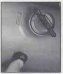
Press the button in to make your front and rear turn signal lamps flash on and off.
