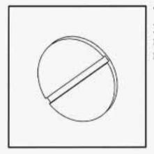
To access the equipment in your wagon, turn the slotted release button located on the rear edge of the cover.
