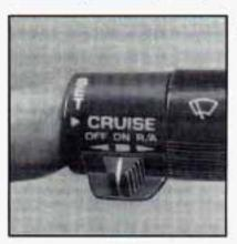
Push in the SET button at the end of the lever and release it.
