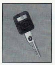
The square key is for the ignition only. It has a bar code attached. Your dealer or qualified locksmith can make extra ignition keys by reading the bar code tag.
