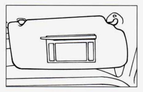
The lighted visor vanity mirror lights up when the mirror cover is opened. Closing the mirror cover turns off the lamps.
