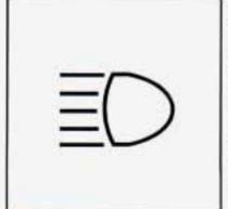
To change the headlamps from low beam to high or high to low, pull the turn signal lever all the way toward you. Then release it. When the high beams are on, this light on the instrument panel will also be on.
