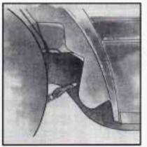
Attach T-hook chains on both sides, in the slotted holes in the side of the frame rails, behind the front wheels.
