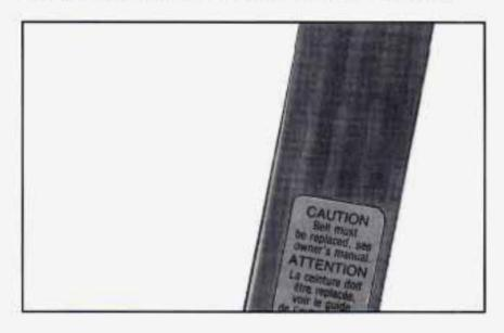
If you ever see a label on the driver's or the right front passenger's safety belt that says to replace the belt, be sure to do so. Then the new belt will be there to help protect you in a collision. You would see this label on the belt near the door opening.
