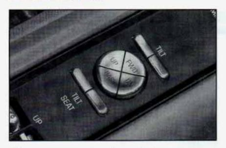
The power seat controls are located on the armrest.
