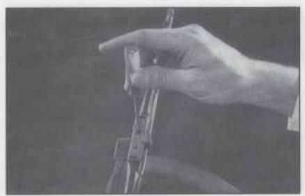
It's a good idea to clean or replace the wiper blade assembly every six months. For the proper windshield wiper blade length and type, see "Replacement Parts" later in this section. To remove the wiper blade assembly:
