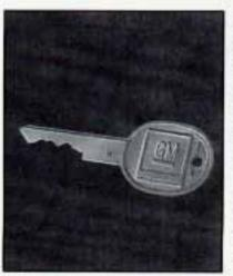
The oval key is for the doors and all other locks. Your door key has a plug. When a new Buick is delivered, the dealer removes the plug from the key, and gives it to the first owner. Each plug has a code on it that tells your dealer or a qualified locksmith how to make extra keys.
