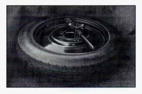
The equipment you'll need is in the trunk if you have a sedan. Turn the wing nut on the screw counterclockwise to remove it. Remove the wheel wrench, spare tire and the jack from the trunk.
