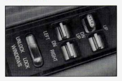
The power windows controls are on the driver's armrest. They control each of the four windows. To open a window, move the switch toward DN. To close it, move the switch toward UP. The switch for the driver's window has an express-down feature. Pull the AUTO switch back all the way. Once engaged, release it and the window will lower all the way. To stop the window from lowering, press the switch forward. To raise the window, press the switch forward.
