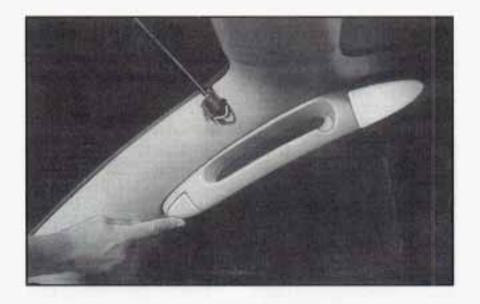
These lamps come on when the tailgate is opened as a door, They turn off when the tailgate is completely closed.
