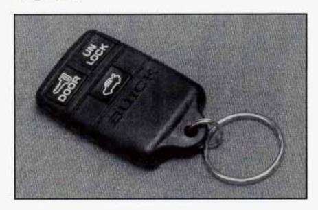
If your Buick has this option, you can lock and unlock your doors or unlock your trunk or tailgate from up to 30 feet (9 m) using the key chain transmitter supplied with your vehicle.
