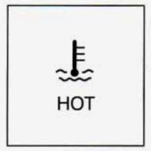
This light comes on as a bulb check when you start your engine. This light tells you that your engine coolant has overheated.
