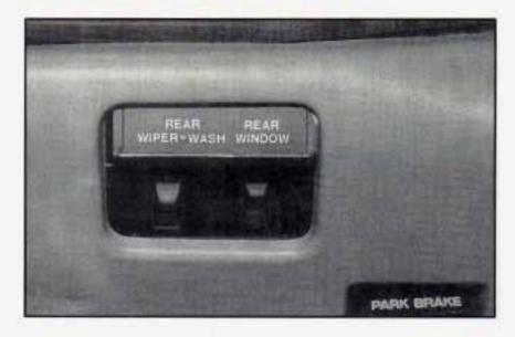
Press the top of the REAR WINDOW switch to unlock the rear window only when the vehicle is in PARK (P) or NEUTRAL (N). You can also unlock the rear window by using the oval key in the lock near the window. This also unlocks the tailgate.
