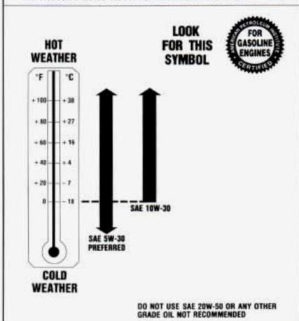
As shown in the chart, SAE 5W-30 is best for your vehicle. However, you can use SAE 10W-30 if it's going to be 0°F (-18°C) or above. These numbers on an oil container show its viscosity, or thickness. Do not use other viscosity oils, such as SAE 20W-50.
