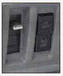
To lock the door from the inside, slide the lock control down.
