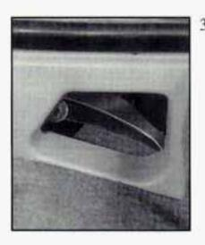
Pull the seat release handle in the lower right corner of the storage compartment. The seatback is now unlocked.
