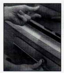
Once the tailgate has been unlocked, you can unlatch the tailgate window by pushing the key cylinder button all the way in. Then raise the window.
