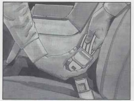
Tilt the latch plate to adjust the belt if needed. 5. Buckle the belt. Make sure the release button is
