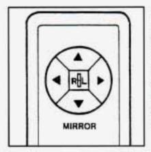
If your Buick has optional power mirrors, the mirror control is located on the driver's door. Move the center switch to choose either side mirror. Press any of the four arrows to move the mirror in the desired direction.
