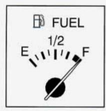
Your fuel gage shows how much fuel is in your tank. It works only when the engine is on. When the indicator nears EMPTY (E), you still have a little fuel left. You need to get more right away.
