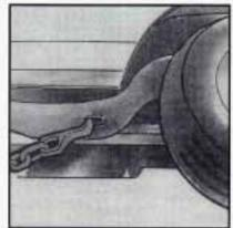
Attach T-hook chains to the slots in the frame rails just ahead of the rear wheels on both sides.
