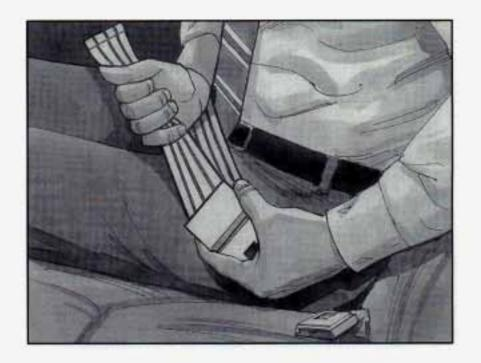
When you sit in a center seating position or in a station wagon third seat, you have a lap safety belt, which has no retractor. To make the belt longer, tilt the latch plate and pull it along the belt.
