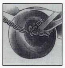
Attach a separate safety chain around the outboard end of each lower control arm.
