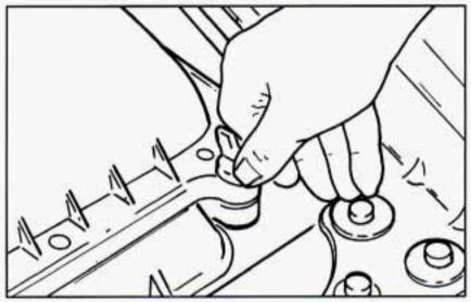
To check or replace the filter, loosen the wing nuts and lift up the cover.
