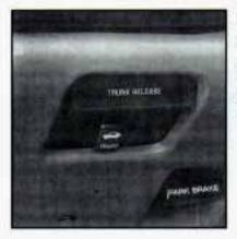
The TRUNK button is to the left of the steering column. Press it to open the trunk from inside your vehicle.
