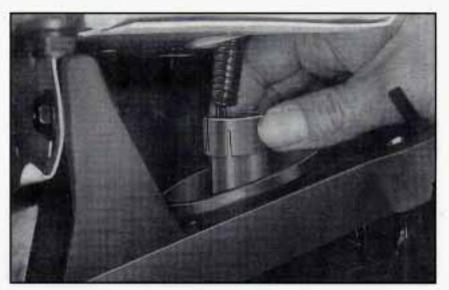
Gently pull the headlamp bulb assembly straight out from the access area.
