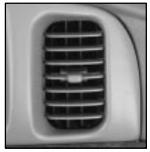
Adjust the direction of airflow by moving the louvered vents.
