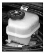
Your brake master cylinder reservoir is on the driver's side of the engine compartment. It is filled with DOT-3 brake fluid. See "Engine Compartment Overview" in the Index.
