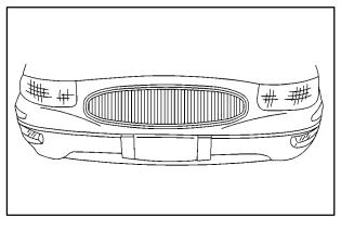
Your vehicle has a visual optical headlamp aiming system equipped with horizontal aim indicators. The aim has been preset at the factory and should need no further adjustment. This is true even though your horizontal aim indicators may not fall exactly on the "0" (zero) marks on their scales.
