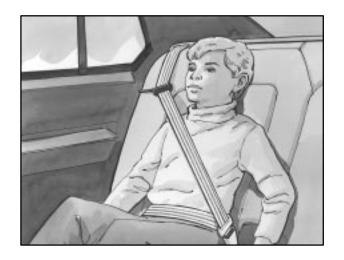
Buckle, position and release the safety belt as described in "Rear Seat Passenger Positions" earlier in this section. Make sure that the shoulder belt crosses the shoulder.
