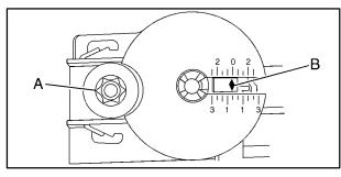
Once the horizontal aim is adjusted, then adjust the vertical aim.
