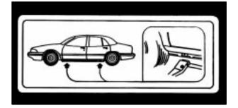
4. Put the jack into a notch in the frame which is located near each wheel well. The front notch is eight inches (20 cm) back from the front wheel well. The rear notch is three inches (8 cm) forward from the rear wheel well. The notches are accessible through openings in the plastic trim at the bottom of the vehicle.
