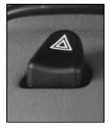
The hazard warning flasher button is located on top of the steering column.
