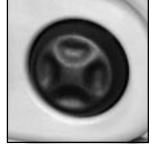
If your vehicle has this feature, the power lumbar control is located on the outboard side of each front seat. Use the power seat control first to get the proper position. Then continue with the lumbar adjustment.
