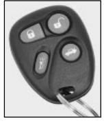
When the unlock symbol is pressed, the driver's door will unlock and the exterior lights will flash twice.
