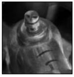
There is one bleed valve. It is located on the thermostat housing.
