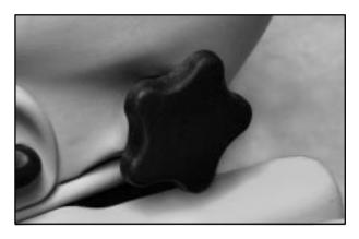
The knob that controls this feature is located on the outboard side of each front seat. Turn the knob toward the front of the vehicle to increase lumbar support. Turn the knob toward the rear of the vehicle to decrease lumbar support.
