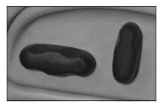
If your vehicle has this feature, the power seat controls are located on the outboard side of each front seat cushion.
