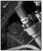
The power steering fluid reservoir is located below the generator and behind the accessory drive belt in the rear of the engine compartment on the passenger's side of the vehicle.
