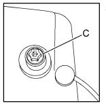
5. Turn the vertical aiming screw (C) until the headlamp beam is aimed to the horizontal tape line.
