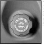
The engine oil fill cap is located near the engine oil dipstick. See "Engine Compartment Overview" in the Index for more information on location.
