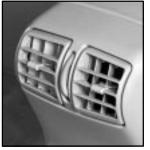
If you have the optional rear passenger ComforTemp, you can adjust the direction of the airflow to the rear seating area.
