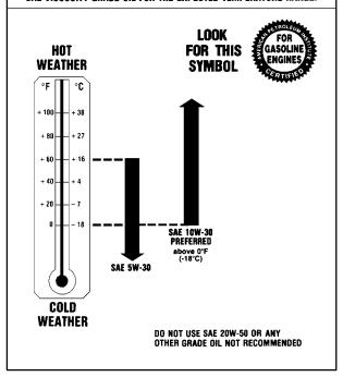
SAE 10W-30 is best for your vehicle. However, you can use SAE 5W-30 if it's going to be colder than 60°F (16°C) before your next oil change. When it's very cold, you should use SAE 5W-30. These numbers on an oil container show its viscosity, or thickness. Do not use other viscosity oils, such as SAE 20W-50.
