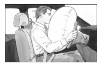
The driver's frontal air bag is in the middle of the steering wheel.
