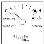
This gage shows the engine coolant temperature. If the pointer moves into the shaded area, the engine is too hot.
