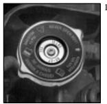
12. Then replace the presure cap. At any time during this procedure if coolant begins to flow out of the filler neck, reinstall the pressure cap. Be sure the arrow on the pressure cap lines up like this.
