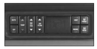
**TEMP** (**Temperature**): To manually adjust the temperature inside the vehicle, push the TEMP arrow. Push the TEMP up arrow for warmer temperature settings and the TEMP down arrow for cooler temperature settings. The setting will be shown in the display. The display will then return to the outside temperature after a few seconds.
