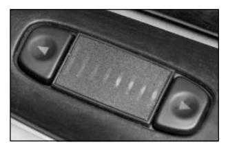
If your vehicle is equipped with the Dual Automatic ComforTemp<sup>™</sup> system, the front seat passenger can control the air temperature in his or her seating area. The control is located on the passenger's door armrest.
