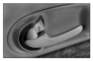
To unlock the door from the inside, move the manual door lock located above the door handle rearward. To lock the door, move the manual door lock forward.
