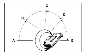
(A) ACCESSORY: This position lets you use your electrical power accessories such as power windows, power sunroof (option), radio and the windshield wipers. To use, push in the ignition key and turn it toward you. Your steering wheel will remain locked, just as it was before you inserted the key.
