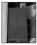
The rear fuse block is located beneath the rear seat on the driver's side. The rear seat cushion must be removed to access the fuse block. See "Removing the Rear Seat Cushion" in the Index.
