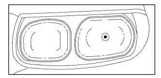
Measure the distance from the ground to the aim dot on each lamp; if left low beam, subtract two inches. Record this distance. 3. At the wall or other flat surface, measure from the ground upward the recorded distance from step 2 and draw or tape a horizontal line the width of the vehicle.
