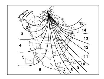
3. Once a zone number appears in the display, press COMPASS (or the on/off button for mirrors equipped with OnStar controls) quickly until the correct zone number appears in the display. Stop pressing the button and the mirror will return to normal operation. If C appears in the compass window, the compass may need calibration. See "Compass Calibration" explained previously.
