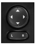
The controls for the power remote mirrors are located on the driver's door armrest.
