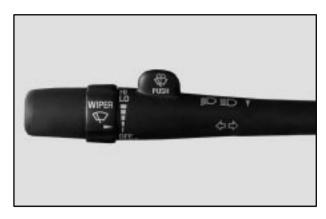
The windshield wipers are controlled by turning the band marked WIPER.
