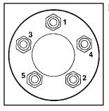
11. Tighten the wheel nuts firmly in a crisscross sequence.
