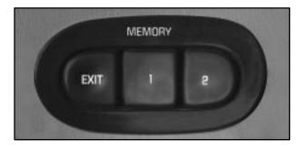
If your vehicle has this feature, the controls are located on the driver's door panel, and are used to program and recall memory settings for the driver's seating, outside mirror positions and comfort controls. See "Comfort Controls" in the Index for more information.
