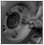
9. Reinstall the wheel nuts with the rounded end of the nuts toward the wheel. Make sure each wheel stud is centered in each wheel hole while tightening the nuts. Tighten each nut by hand until the wheel is held against the hub.
