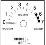
The tachometer tells you how fast the engine is running. It displays engine speed in thousands of revolutions per minute (rpm).
