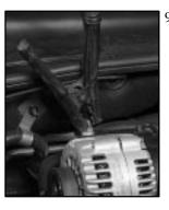
of the negative (-) cable at least 18 inches (45 cm) away from the dead battery, but not near engine parts that move. The electrical connection is just as good there, and the chance of sparks getting back to the battery is much less.
