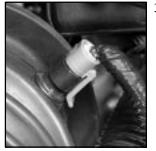
3. Disconnect the electrical connector from the air intake hose. This will allow you to lift the rear portion of the engine air cleaner/filter housing.
