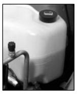
The engine coolant recovery tank is located in the engine compartment on the passenger's side of the vehicle. See "Engine Compartment Overview" in the Index for more information on location.
