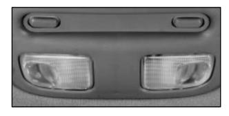
The front reading lamps, located on the headliner, are turned on or off by pressing one of the buttons located near each lamp.
