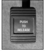
This vehicle has a PUSH TO RELEASE parking brake pedal. To set the parking brake, hold the regular brake pedal down with your right foot. Push down the parking brake pedal with your left foot.
