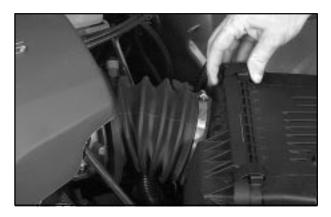
1. Lift the latches on the engine air cleaner/filter housing cover.
