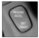
The switches to operate cruise control are located on the steering wheel.
