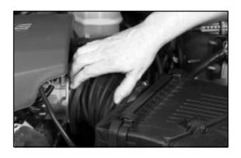
2. Remove the air intake hose that is snapped over the throttle body by pulling the hose upward and away from the throttle body which is located near the top of the engine.
