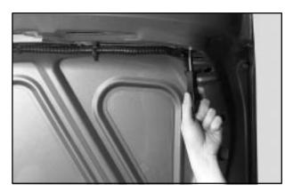
1. Loosen and remove the seven fasteners that hold the assembly in place. The assembly for both sides is one piece. The entire piece must be removed to replace any bulbs.
