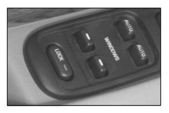
The power window controls located on the driver's door armrest operate each of the windows while the ignition is on or while Retained Accessory Power (RAP) is active. In addition, each passenger door has a control for its own window. See "Retained Accessory Power (RAP)" in the Index for more information.
