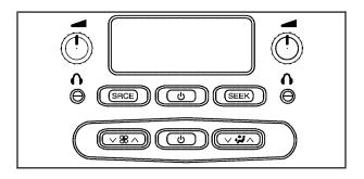
() (Power): Press this button to turn the system on or off. The rear speakers will be muted when the power is turned on.
