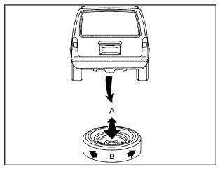
6. Make sure the tire is stored securely. Push, pull (A), and then try to turn (B) the tire. If the tire moves, use the wheel wrench and socket end of the extension to tighten the cable.
