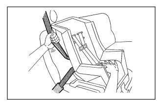
6. To tighten the belt, push down on the child restraint, pull the shoulder portion of the belt to tighten the lap portion of the belt and feed the shoulder belt back into the retractor. If you are using a forward-facing child restraint, you may find it helpful to use your knee to push down on the child restraint as you tighten the belt. You should not be able to pull more of the belt from the retractor once the lock has been set.
