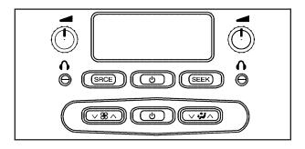
$V \% \land$  (Fan) Press this button to adjust the fan speed.
