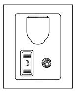
The accessory inflator is located in the rear compartment on the driver's side of the vehicle behind an access cover, near the liftgate opening.
