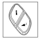
**(Trip Information):** Press this button to display the odometer, trip odometers, and timer.
