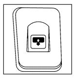
Press and release the back of the control in the overhead console to open the sunroof. Press the front of the control to close the sunroof.
