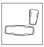
The power seat controls are located on the outboard side of the front seat cushions. The horizontal control adjusts the seat cushion and the vertical control adjusts the seatback.
