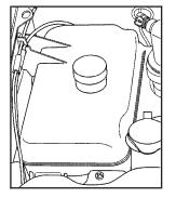
The coolant level should be at least up to the FULL COLD mark. If it is not, you may have a leak at the pressure cap or in the radiator hoses, heater hoses, radiator, water pump, or somewhere else in the cooling system.
