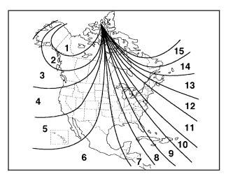
Press the COMP button on the bottom of the mirror until the new zone number appears in the display. After you stop pressing the button, the display will show a compass direction within a few seconds.
