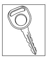
This vehicle has one double-sided key for the ignition and door lock. It will fit with either side up.
