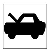
To open the hood, first pull the handle with this symbol on it. It is located inside the vehicle under the instrument panel on the driver's side.
