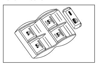
The controls for the power windows are located on the armrest on each of the side doors. With power windows, the switches operate the windows when the ignition is in RUN, ACCESSORY or when Retained Accessory Power (RAP) is active. See *Retained Accessory Power (RAP)* on page 2-18. The driver's door also has a switch for each of the passenger's windows.
