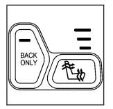
Your vehicle may have heated front seats. The buttons used to control this feature are located on the front door armrests. The engine must be running for the heated seat feature to work.
