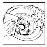
Remove any rust or dirt from the wheel bolts, mounting surfaces and spare wheel. 8. Place the spare tire on the wheel-mounting surface.
