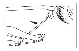
Raise the vehicle by turning the jack handle clockwise. Raise the vehicle far enough off the ground so there is enough room for the spare tire to fit.
