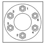
12. Use the wrench to tighten the wheel nuts firmly in a crisscross sequence as shown.
