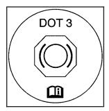
Your brake master cylinder reservoir is filled with DOT-3 brake fluid. See Engine Compartment Overview on page 5-12 for the location of the reservoir.
