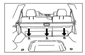
Do not secure a child restraint in the right front passenger's position or in the third row seating position, if the vehicle has one, if a national or local law requires that the top tether be attached, or if the instructions that come with the child restraint say that the top tether must be attached. There is no place to attach the top tether in this position.
