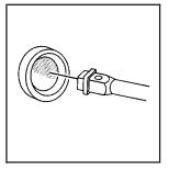
11. If the spare tire is hanging from the cable, insert the socket end of the extension connected to the wheel wrench into the hoist shaft hole just above the rear bumper on a 45 degree angle downward.
