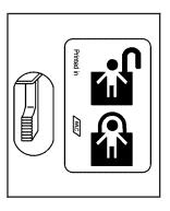
Move the lever down to engage the security lock. Move the lever up to disengage the security lock.
