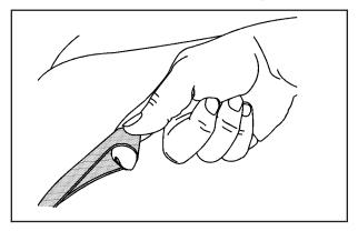
Pull up on the loop located where the seat cushion meets the seatback to fold the seat cushion up and out of the way. This will allow the seatbacks to fold flat and increase the cargo area.
