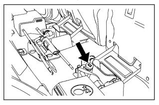
To release the jack from its holder, turn the knob on the jack counterclockwise to lower the jack head.
