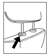
Pull the head restraint up to raise it. Press the release button, located at the base of the head restraint, and push the head restraint down to lower it.
