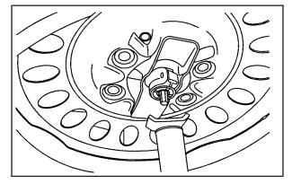
Attach the jack handle, extension(s) and the wheel wrench to the jack and place it under the vehicle towards the front of the rear bumper. Position the center lift point of the jack under the center of the spare tire.
