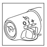
Your vehicle has cruise control. The controls are located on the end of the turn signal/ multifunction lever.
