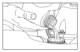
Fill the radiator with the proper DEX-COOL®
