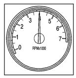
The tachometer displays the engine speed in revolutions per minute (rpm).
