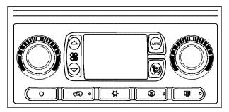
With this system you can control the heating, cooling and ventilation for your vehicle. When your vehicle is first started and the climate control system is on, or if the climate control system has been turned on, the display will show the driver's temperature setting for five seconds. Then it will show the outside temperature.
