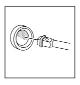
Insert the socket end of the extension (C) on a 45 degree angle downward into the hoist drive shaft hole. It is exposed when the rear gate is open and is just above the rear bumper.
