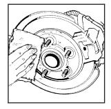
Remove any rust or dirt from the wheel bolts, mounting surfaces and spare wheel. 10. Install the compact spare tire.
