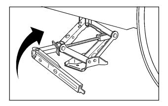
Turn the jack handle clockwise to raise the vehicle. Raise the vehicle far enough off the ground for the compact spare tire to fit under the vehicle.
