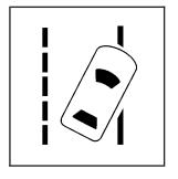
For vehicles with the lane departure warning system, this light briefly comes on green, while starting the vehicle, to indicate that it is working.
