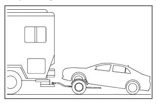
The vehicle can be towed using a dolly. To tow the vehicle using a dolly, follow these steps:
