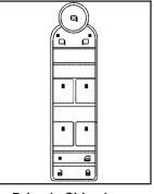
The power window switches are located on the driver's door armrest. In addition, each door has a switch for its own window.
