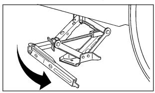
Lower the vehicle by turning the jack handle counterclockwise. Lower the jack completely.
