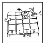
Fill the coolant surge tank with the proper mixture to the FULL COLD mark on the side of the coolant surge tank.
