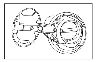
The tethered fuel cap is located behind a hinged fuel door on the driver side of the vehicle. If the vehicle has E85 fuel capability, the fuel cap will be yellow and state that E85 or gasoline can be used. See *Fuel E85* (85% Ethanol) on page 5-8.
