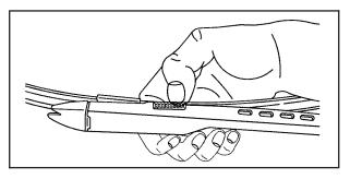
Squeeze the tabs on each side of the wiper blade assembly and slide the assembly off the end of the wiper arm.
