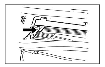
Insert the new air filter by pushing until you hear a click. Reinstall the push pin and snap the cover into place.
