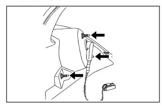
Remove the three hex nuts holding the taillamp assembly in place.
