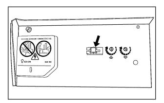
Locate in the garage, the garage door opener receiver (motor-head unit). Locate the "Learn" or "Smart" button. It can usually be found where the hanging antenna wire is attached to the motor-head unit and may be a colored button. Press this button. After pressing this button, complete the following steps in less than 30 seconds.
