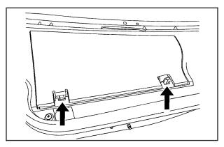
Insert a tool behind the push pin located on the inboard side of the air filter compartment to carefully pry the pin out.
