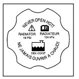
You can remove the pressure cap when the cooling system, including the pressure cap and upper radiator hose is no longer hot. Turn the pressure cap slowly counterclockwise.
