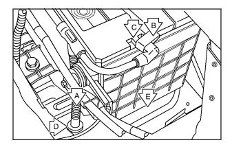
To be sure the vent hose (A) is properly attached, the vent hose connectors (B) must be securely reattached to the vent outlets (C) on each side of the battery and the vent assembly grommet (D) must be secured to the floor pan (E).
