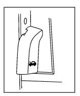
Pull the hood release handle inside the vehicle. It is located next to the parking brake pedal near the floor.
