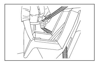
5. Pull the rest of the shoulder belt all the way out of the retractor to set the lock.
