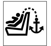
To assist you in locating the top tether anchors, the top tether anchor symbol is located on the cover.
