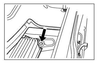
3. To remove the air filter, insert a tool between the air filter and the compartment wall on the outboard side of the vehicle. Then, push in to flatten the pin holding the air filter in place. Gently remove the air filter and any loose debris that may be inside the air filter compartment.
