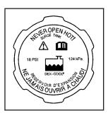
You can remove the coolant surge tank pressure cap when the cooling system, including the coolant surge tank pressure cap and upper radiator hose, is no longer hot.
