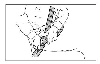
To unlatch the belt, push the button on the buckle. The belt should return to its stowed position. Slide the latch plate up the safety belt webbing when the safety belt is not in use. The latch plate should rest on the stitching near the guide loop on the side wall.
