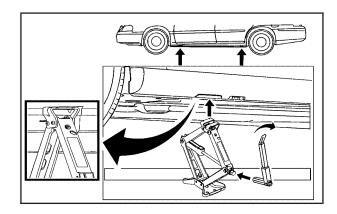
4. Put the jack into the flange in the frame which is located near each wheel well. The flanges are accessible through openings in the plastic trim at the bottom of the vehicle. The front opening is about 8 inches (20 cm) back from the front wheel well. The rear opening is about 3 inches (8 cm) forward from the rear wheel well.
