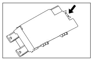
To access the fuse block, pull out and lift up on the cover latch, located at the end of the fuse block, near the battery cable.
