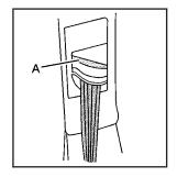
Press the release button (A) and move the height adjuster to the desired position. The adjuster can be moved up by pushing up on the shoulder belt guide.
