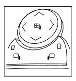
Controls for the outside power mirrors are located on the driver's door armrest.
