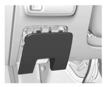
The instrument panel fuse block is in the instrument panel, on the driver side of the vehicle. To operate the fuses, open the fuse panel by pulling down at the top.
