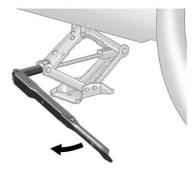
Raise the vehicle by turning the jack handle clockwise. Raise the vehicle far enough off the ground so there is enough room for the road tire to clear the ground.
