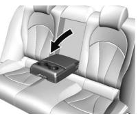
The rear seat has an armrest in the center of the seatback. Lower the armrest to access the two cupholders and the storage area.
