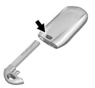
1. Press the button on the transmitter to remove the key.
