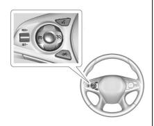
${}^{\scriptsize \mbox{\scriptsize $\Theta$}}$  : Press to turn cruise control on or off. A white indicator comes on in the instrument cluster.
