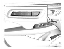
If equipped, the SET, 1, 2, and the (Exit) buttons on the driver door are used to manually store and recall memory settings for the driver seat. The driver memory buttons also store outside mirror, and power tilt and telescoping steering wheel positions (if equipped).
