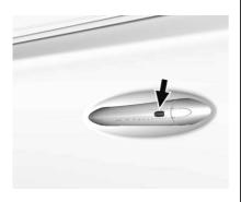
Pressing the lock/unlock button will cause all doors to lock if any of the following occur:
