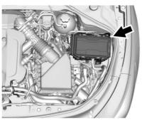
To remove the fuse block cover, squeeze the three retaining clips on the cover and lift it straight up.
