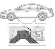
Position the jack lift head at the jack location nearest the flat tire. The location is indicated by a notch in the vertical bottom edge of the body side sheet metal. The notches in the jack must align with the notch in the rocker pinch weld. The jack lift head lifts on the inward side of the pinch weld flange.
