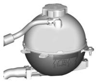
Check to see if coolant is visible in the coolant surge tank. If the coolant inside the coolant surge tank is boiling, do not do anything else until it cools down. If coolant is visible but the coolant level is not at the indicated level mark, wait until the system has fully cooled down, then add a 50/50 mixture of clean, drinkable water and DEX-COOL coolant at the coolant surge tank until the level reaches the indicated level mark. See *Engine Overheating*  $\Leftrightarrow$  238.
