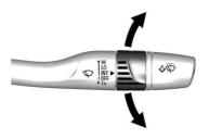
**INT :** Use for intermittent wipes. To adjust wipe frequency, turn the band up for more frequent wipes or down for less frequent wipes.
