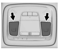
The front reading lamps are in the overhead console.
