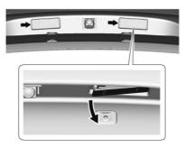
Push the lamp assembly toward the center of the vehicle, then move the lamp downward, and remove it from the vehicle body.
