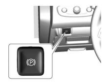
The Electric Parking Brake (EPB) can always be activated, even if the ignition is off. To prevent draining the battery, avoid repeated cycles of the EPB when the engine is not running.
