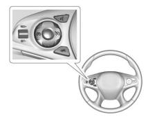
O: Press to turn cruise control on or off. A white indicator comes on in the instrument cluster.
