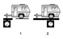
The trailer tongue (1) should weigh 10 % of the total loaded trailer weight (2).
