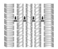
Treadwear indicators are one way to tell when it is time for new tires. Treadwear indicators appear when the tires have only 1.6 mm (1/16 in) or less of tread remaining. See *Tire Inspection*  $\Leftrightarrow$  266 and *Tire Rotation*  $\Leftrightarrow$  266.
