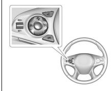
$\mathfrak{S}$ : Press to turn the system on or off. The indicator turns white on the instrument cluster when ACC is turned on.
