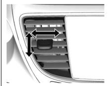
Use the slider knob on the air vent louvers to change the amount and direction of the airflow.
