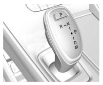
The shift pattern is displayed in the top of the shift lever. The selected gear position will illuminate red on the shift lever, while all others will be displayed in white. If the shift is not immediate, as in very cold conditions, the indicator on the shift lever may blink until it is fully engaged. The shift lever always starts from a center position, represented by an amber dot on the shift pattern. After releasing the shift lever, it will return to the center position.
