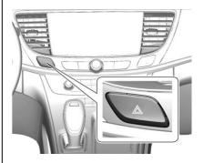
$\triangle$ : Press to make the front and rear turn signal lamps flash on and off. Press again to turn the flashers off.
