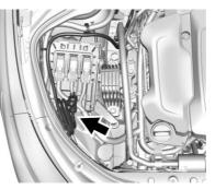
The electrical cord is on the driver side of the engine compartment, between the fender and the engine compartment fuse block.
