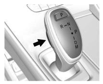
This vehicle is equipped with an electronic transmission. The shift lever unlock button is designed to prevent inadvertent shifting out of P (Park) unless the ignition is in ON/RUN, the brake pedal is applied, and the shift lever unlock button is pressed.
