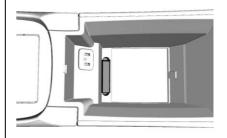
4. Place the new transmitter into the transmitter pocket inside the armrest storage area.
