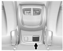
The vehicle may have a power outlet that can be used to plug in electrical equipment with a maximum limit of 150 watts. The power outlet is on the rear of the center console.
