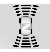
The instrument cluster may have a Parking Assist display with bars that show "distance to object" and object location information for RPA, and on some vehicles, FPA. As the object gets closer, more bars light up and the bars change color from yellow to amber to red.
