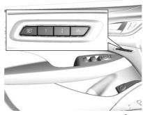
If equipped, the SET, 1, 2, and (Exit) buttons on the driver door are used to manually store and recall memory settings for the driver seat. The driver memory buttons also store outside mirror, and power tilt and telescoping steering column (if equipped) positions.
