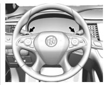
Vehicles with Tap Shift have controls on the back of the steering wheel to manually shift the automatic transmission.
