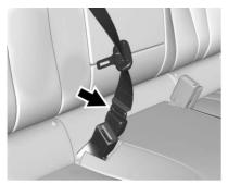
2. Disconnect the rear safety belt mini-latch, using a key in the slot on the mini-buckle.
