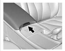
Push the storage compartment lid backward and pull up to open the storage compartment lid. Two USB ports and an auxiliary jack are inside.
