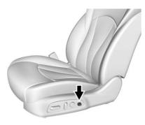
If equipped, press the massage button to use the massage feature. To stop massage, press this button again.
