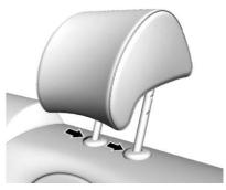
2. Press both buttons on the head restraint posts at the same time, and pull up on the head restraint.
