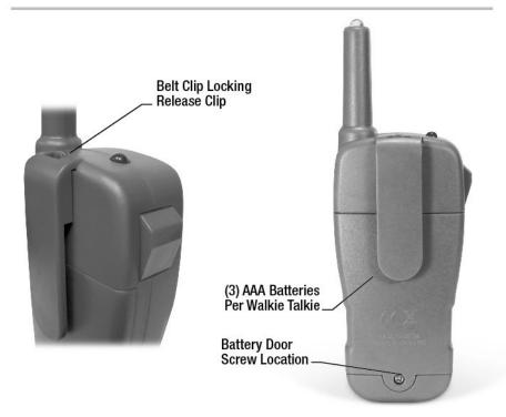
To install the batteries release the belt clip locking clip and slide the belt clip vertically off the back of the walkie talkie body. Remove the battery compartment screw and lift the battery door off. Insert (3) AAA batteries as shown in illustration. Replace battery door and secure with screw. Replace belt clip and ensure it's secure.
