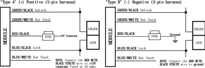
NOTE: Once you have made the connections for the 5-pin door lock harness, you will need to plug the door lock harness into the main module 5-pin plug on the front of the unit.
