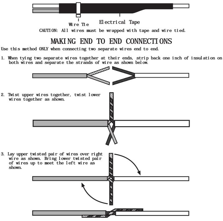
4. Use electrical tape to wrap, be sure to cover about 2 inches on either side of connection. Secure with wire ties as shown. Electrical Tape
