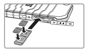
4. Insert the SIM tray into the SIM card slot.
