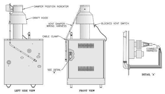
Figure 7: Plug-in Damper Installation
