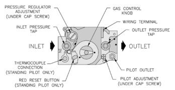
Figure 19: Top View of VR Gas Valves
