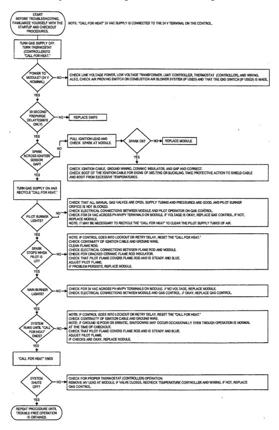
Figure 28: Troubleshooting Guide, Honeywell Electronic Ignition (EI)
