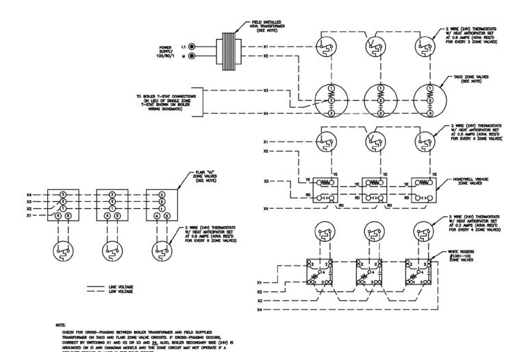
Figure 15: Wiring Schematic, Zone Valves
