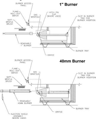
Figure 30: Burner Cleaning and Installation
