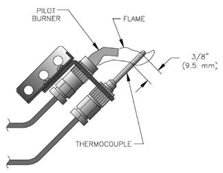
Figure 25: Typical Pilot Flame, Honeywell Q350
