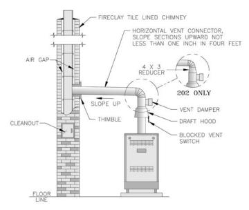
**Figure 8: Typical Vent Installation**
