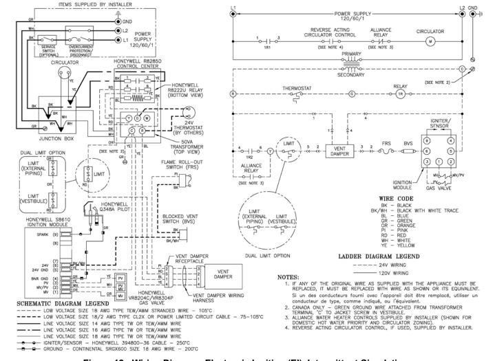
Figure 12: Wiring Diagram, Electronic Ignition (EI), Intermittent Circulation
