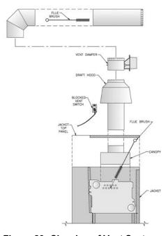
Figure 29: Cleaning of Vent System and Boiler Flues
