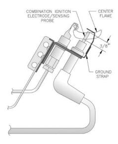
Figure 27: Typical Pilot Flame, Honeywell Q348A
