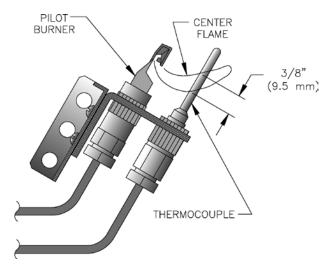
Figure 26: Typical Pilot Flame, Honeywell Q327
