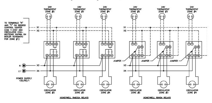
Figure 16: Wiring Schematic, Zone Circulators
