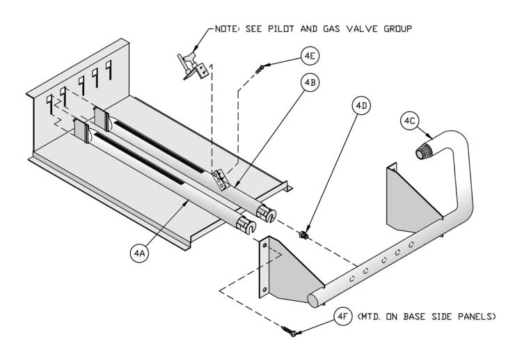
Manifold and Main Burners (1 Inch Main Burners)
