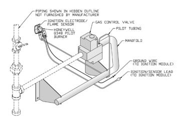
Figure 18: Schematic Pilot and Gas Piping Electronic Ignition (EI)
