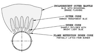
Figure 23: 40mm Main Burner Flame
