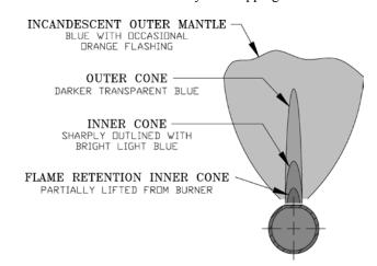
Figure 24: 1 Inch Main Burner Flame
