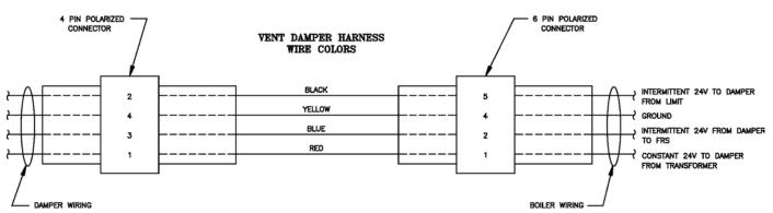
Figure 9: Vent Damper Schematic Wiring Diagram
