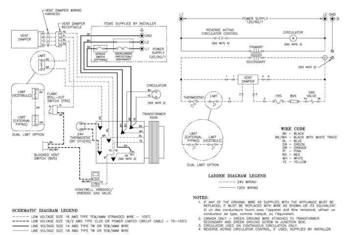
Figure 13: Wiring Diagram, 24 Volt Standing Pilot with Continuous or Gravity Circulation
