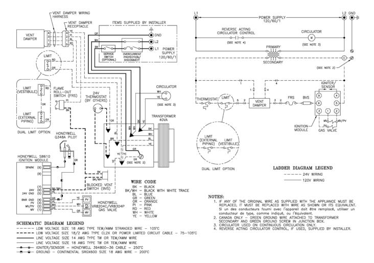
Figure 14: Wiring Diagram, Electronic Ignition (EI), Continuous or Gravity Circulation
