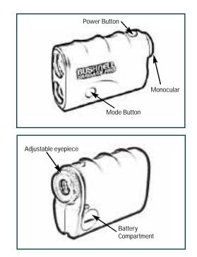
Standard (LCD Indicator - none) This setting allows most targets to be distanced up to 570 yards. Used for moderately reflective targets that are typical of most distancing situations. The minimum distance in the standard mode is 10 yards.
