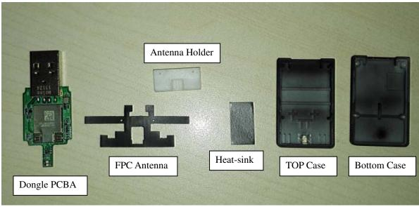
**Step 1**: Paste FPC antenena to antenna holder to construt the antenta pattern as the picture showns at below:
