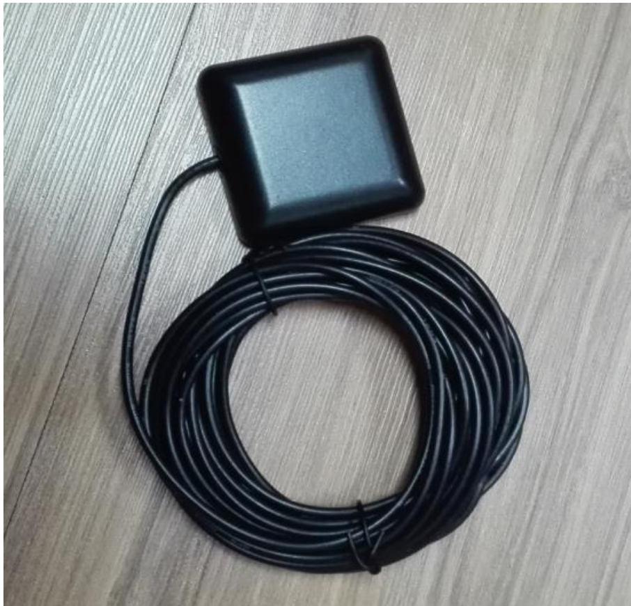
Figure 31 Image of GPS Antenna from Top view
