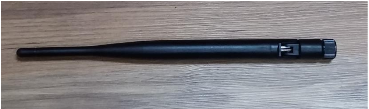
Figure 45 Image of V2X Antenna2 (SMA rotate 0 degree)
