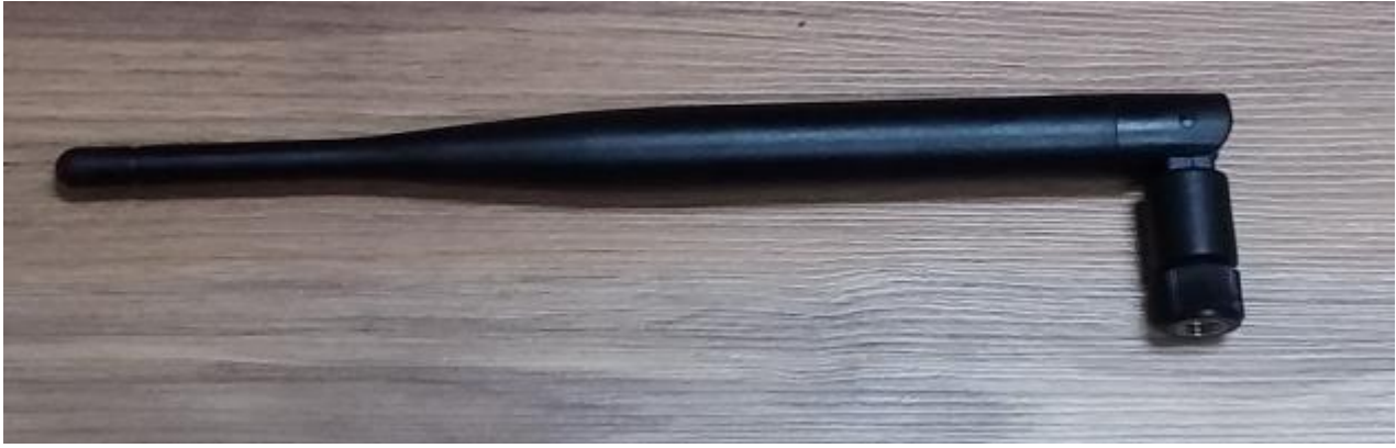
Figure 44 Image of V2X Antenna2 (SMA rotate 90 degree)
