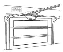
For overhead garage door mounting, mount the sensor near the top of the door with the tilt sensor facing down as shown
