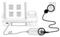
Connect the ADSL modem cable, cable modem or LAN cable to the IP Videophone.
