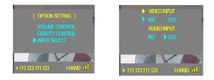
① VIDEO INPUT: If you select 'INT' from A/V Input menu, you can insert an image through the camera of IP videophone, but if you choose 'EXT', an image is inserted from the external camera connected to video input terminal of backside of the videophone body.
