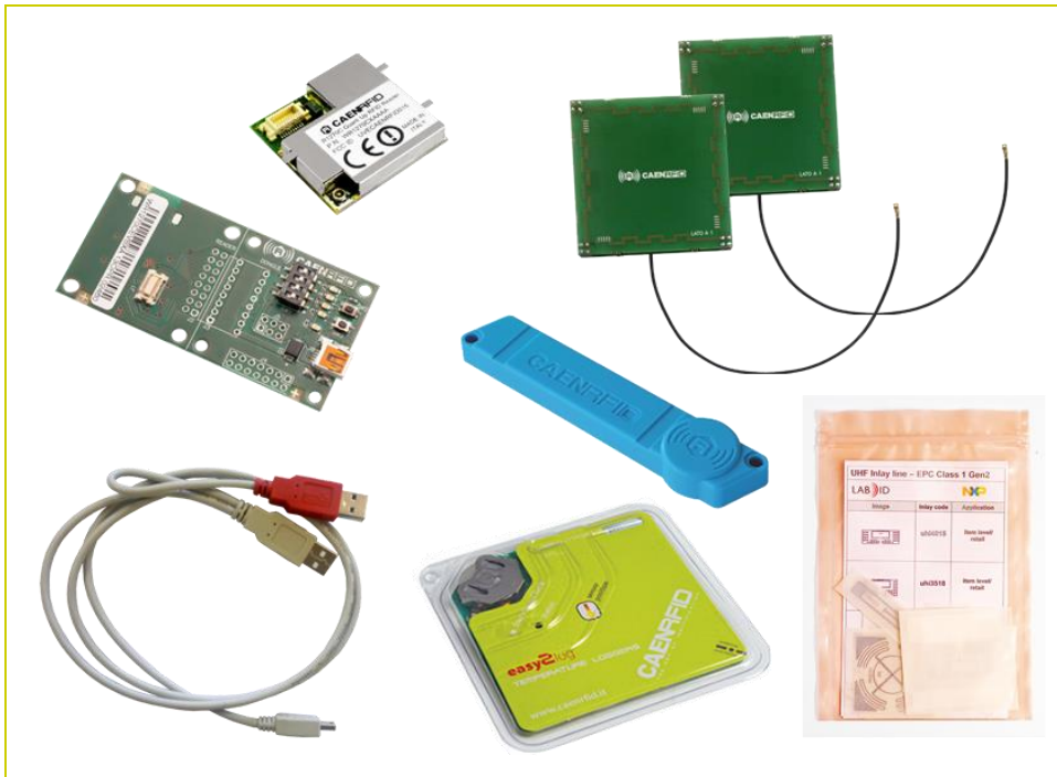
Fig. 1.4: R1270CXDK: R1270 - Development kit with reader, adapter, antennas, cable and demo tags
