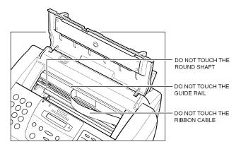
4. Use a clean, soft, dry, lint-free cloth to remove any ink or paper debris from the unit's interior, especially around the platen. Be careful not to touch the BJ cartridge.
