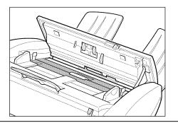
7. When you are finished, close the operation panel by pressing it down from the center as shown.
