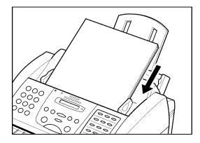
The document is now ready for scanning. The MultiPASS automatically feeds the pages one by one from the bottom of the stack.
