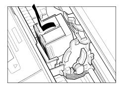
7. Peel the cover off the new BJ cartridge's protective packaging, and remove the BJ cartridge.
