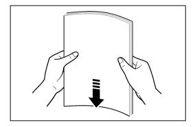
2. "Slant" the stack so that its front edge is bevelled as shown below, then insert the stack into the ADF.
