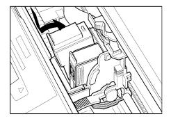
9. Press firmly on the tab on top of the new ink tank, in the direction shown below, until the tank snaps into place.
