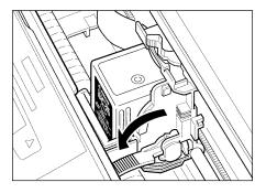
The BJ cartridge is now locked into position.
