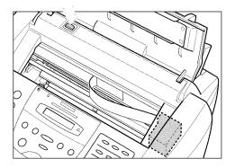
The cartridge holder moves to the center of the unit.
