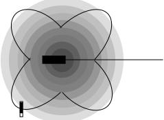
(B) When antenna and tag are perpendicular with each other<Fig. 9> Recognition distance (Read) in accordance with arrangement of antenna and tag
