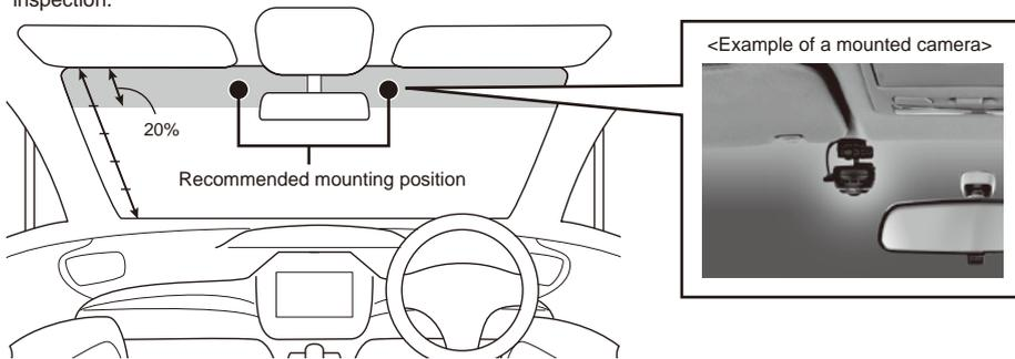
**CAUTION** When mounting the camera, ensure to meet all the below requirements.
