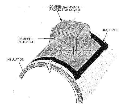
Fig. 1—Damper Actuator Protective Cover
