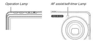
\* There are three lamp flash patterns. Pattern 1 flashes once per second, Pattern 2 flashes twice per second, and Pattern 3 flashes four times per second. The table below explains what each flash pattern indicates.
