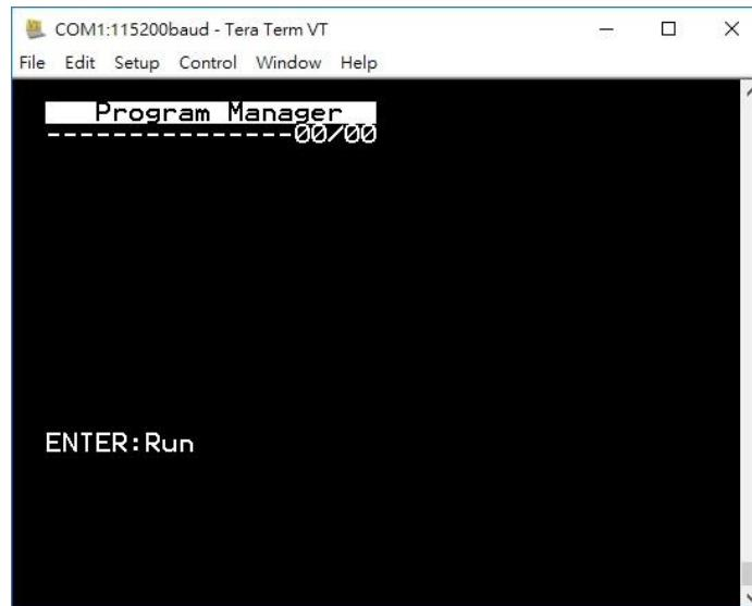
Once the power is on in normal status, UPT1000B will enter Program Manager if no default application selected. All user applications are listed in Program Manager. User can select an application and run the application, view the application info, delete the application, or set application to the default one to run once the power is on. Users may enter System Menu to configure UPT1000B settings.
