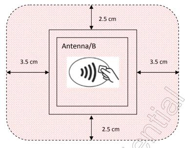
3D: Any metal or conductive material is forbidden in the operating volume shown as below.
