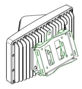
(3) Use screws to secure the two plates together as shown below. Screws #4 should be torqued to a maximum of 5 ft-lbs (69 kgf-cm). (NOTE: IBR is shown inverted from the way it should be mounted.)
