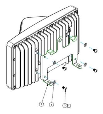
(2) Attach the pole bracket to the plate on IBR using the hooks as shown in the next two diagrams. NOTE: If IBR will be attached to a wall, the pole bracket should be turned so that the pole side faces IBR and the flat side faces outward.
