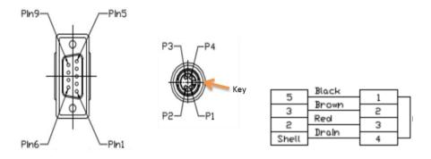
This interface can be used by an operator only to control, configure, and troubleshoot IBC, but not for general network connectivity or data transmission. Pin-outs of the four-pin serial connector are shown in the table below.
