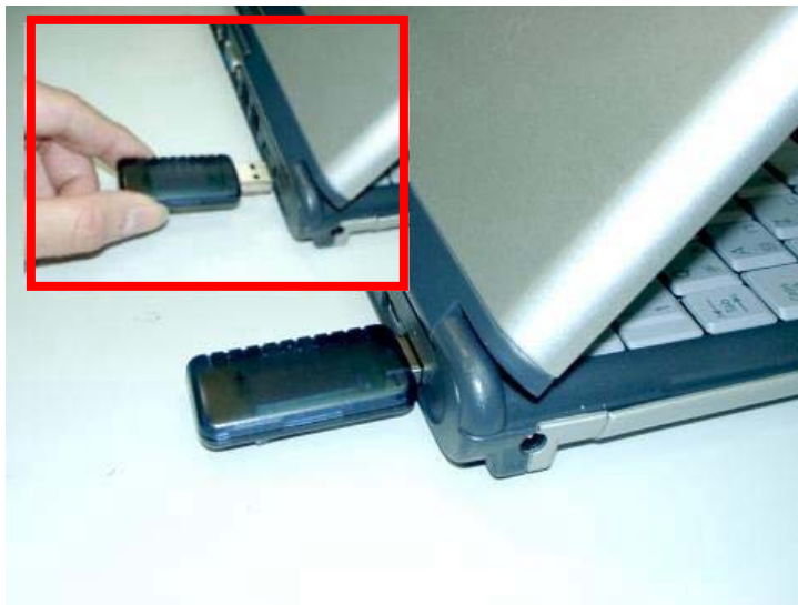
Figure 2-10: Plug the Bluetooth USB Adapter into USB port on laptop PC
