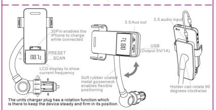
Turning on the Unit Insert the Cigarette plug on IT-0822 into the Car Cigarette Lighter socket, spin the lock on the plug to make sure that position is locked. Flex the gooseneck into a position that is suitable for you to use. Place the unit onto the clamp of IT-0822 and connect the 3.5mm Aux cable. Once you start up the car, IT-0822 will be automatically turned on.
