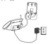
1 Insert the four tabs on the wall mount into the four slots on the back of the base then push down.
