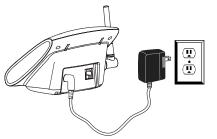
Rest the handset in the base so the in use/charge LED lights. Charge the battery for at least 12 hours. Do not plug the phone into the phone jack until the battery is fully charged.
