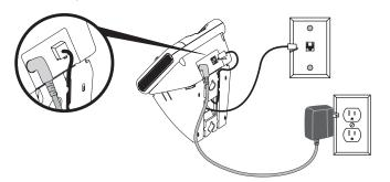
O Line up the tabs on the wall mount bracket with the holes on the back of the wall mount. Snap the wall mount firmly into place.
