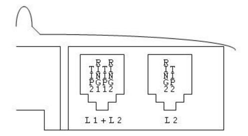
If your telephone outlet is wired for 2 lines then connect a single 4-conductor TELCO line between the telephone outlet and the "L1 + L2" jack on back of the base.
