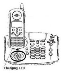
**6** For the initial charge, charge the battery for at least **16** hours.
