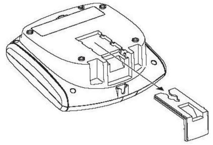
**2** Turn the wall mount over so the key slot is facing upward. Alight the holes of the wall mount with the feet of the base and push gently until the wall mount fits snugly into place.
