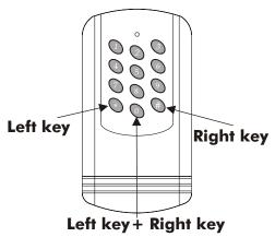
During a dial phase, the key "\*" has the functionality of a backspace. It can be used to correct a wrong dialing. Once finished the number dialing, the key "\*" goes back to the standard functionality corresponding to the LEFT key of a Master transmitter.
