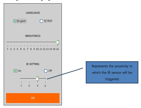
Under IR/Brightness/Language, you can toggle the language between English and Korean, adjust the brightness of the display, or change the distance of detection for the IR sensor.
