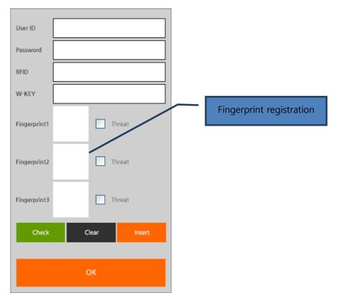
You can register a new user by accessing the 'User Registration Screen' from setting. By default, User ID and Password are mandatory and need to be inserted to register a new user.
