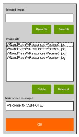
You can modify the images that are displayed on the slide-show via this page. Currently, a maximum of 4 images can be saved. Each image must be less than 100kB.
