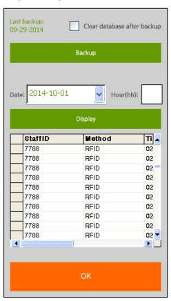
In 'Log Management', you can back-up or view all the attempted access made via the device. By clicking 'Backup', you can save the logs in .csv format (which can be open using Microsoft Excel or any relevant software).
