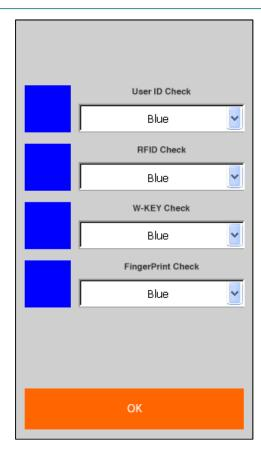
Any same color chosen for the authentication methods only require user to provide either one of them for successful authentication. For example, the combination such as the image above require users to provide only one type of authentication for successful authentication.
