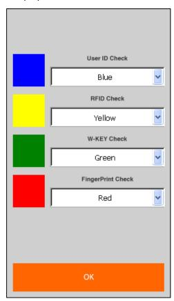
There are four colors currently available for choosing as shown in the image above. If a combination like the image above is chosen, users must provide all four methods of authentication (regardless of sequence) to achieve a successful authentication.
