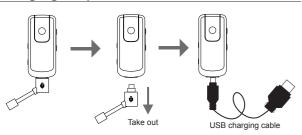
Take out the mic connector and put in the charging cable connector for battery recharging.
