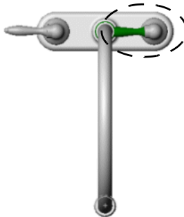
Collision detection without Stop at Collision active. Notice the handle moves inside the spigot.
