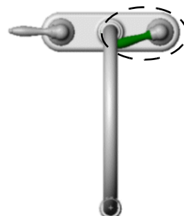
Collision detection with Stop at Collision active. Notice the handle cannot move inside the spigot.
