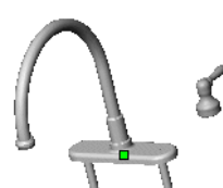
Dragging the second handle component into the assembly
